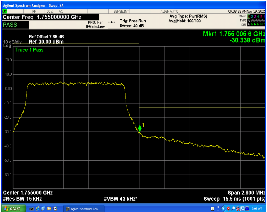
Band4 QAM16 BW=10MHz Channel=20000 RB Size=1 Position=#0
