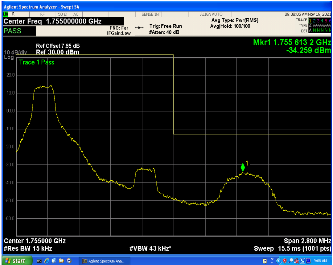
Band4 QPSK BW=1.4MHz Channel=20393 RB Size=1 Position=#Max
