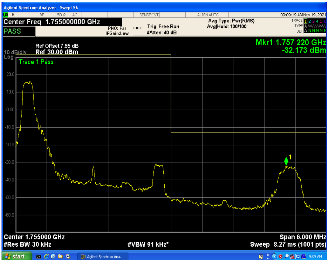
Band4 QAM16 BW=5MHz Channel=19975 RB Size=1 Position=#0
