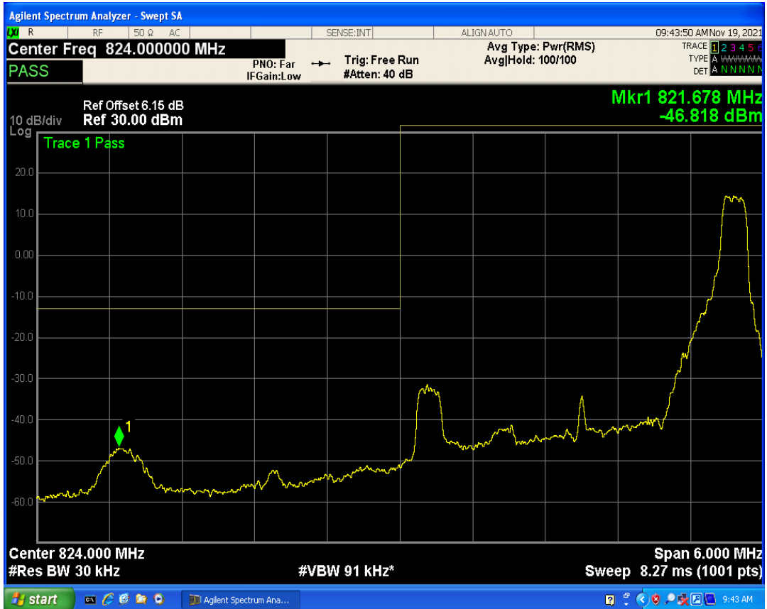
Band5 QAM16 BW=10MHz Channel=20600 RB Size=50 Position=#0
