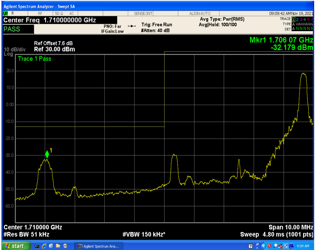
Band4 QPSK BW=5MHz Channel=19975 RB Size=25 Position=#0
