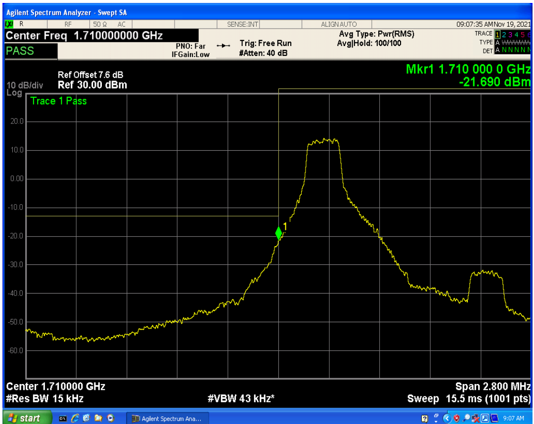
Band4 QAM16 BW=5MHz Channel=20375 RB Size=25 Position=#0
