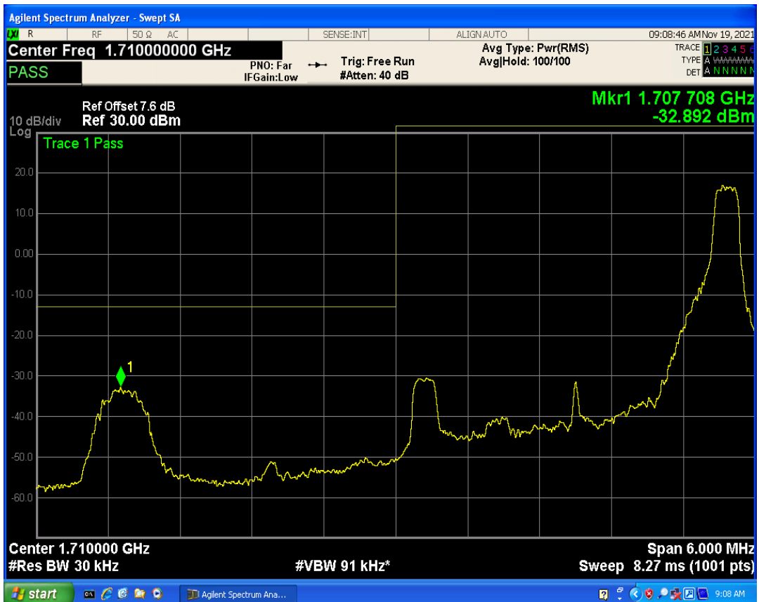
Band4 QPSK BW=5MHz Channel=19975 RB Size=1 Position=#Max
