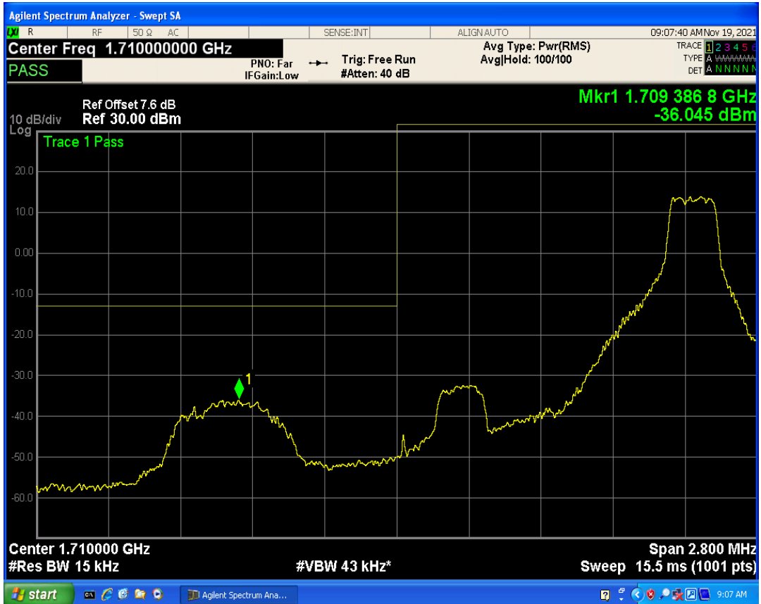
Band4 QPSK BW=1.4MHz Channel=19957 RB Size=6 Position=#0
