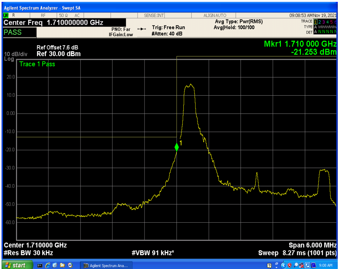
Band4 QAM16 BW=20MHz Channel=20300 RB Size=100 Position=#0
