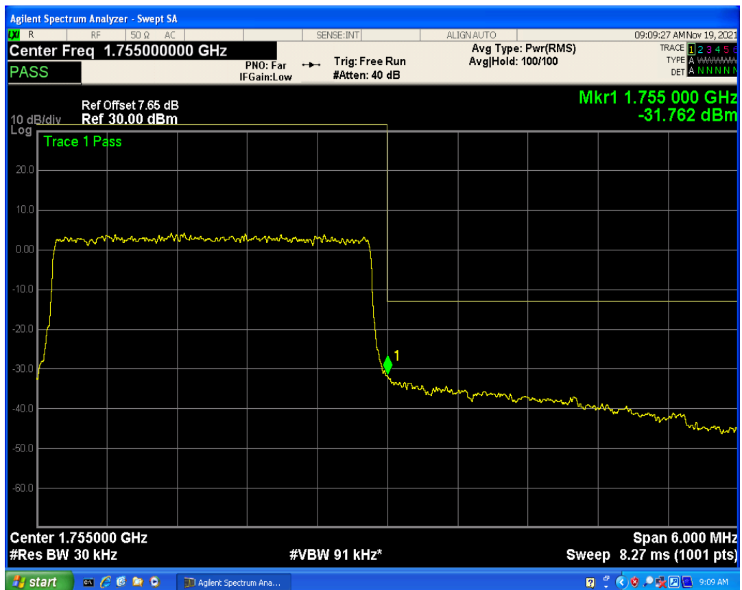
Band4 QAM16 BW=5MHz Channel=20375 RB Size=1 Position=#0
