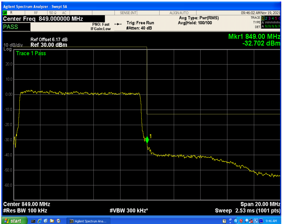
Band5 QAM16 BW=3MHz Channel=20415 RB Size=1 Position=#0
