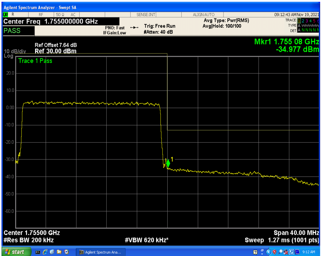
Band4 QAM16 BW=20MHz Channel=20050 RB Size=100 Position=#0
