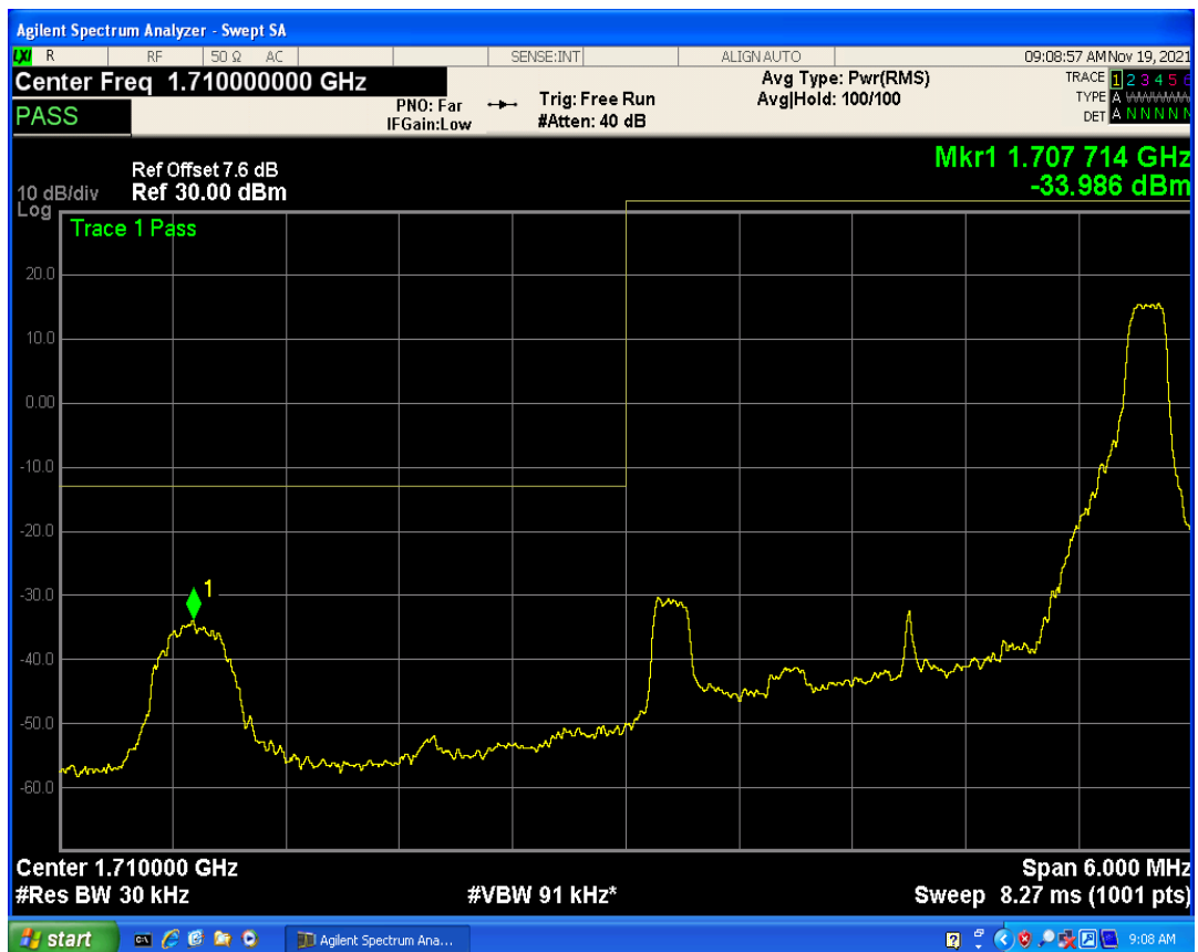
Band4 QAM16 BW=3MHz Channel=20385 RB Size=1 Position=#Max
