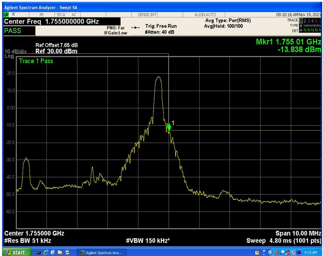
Band4 QPSK BW=1.4MHz Channel=20393 RB Size=1 Position=#0
