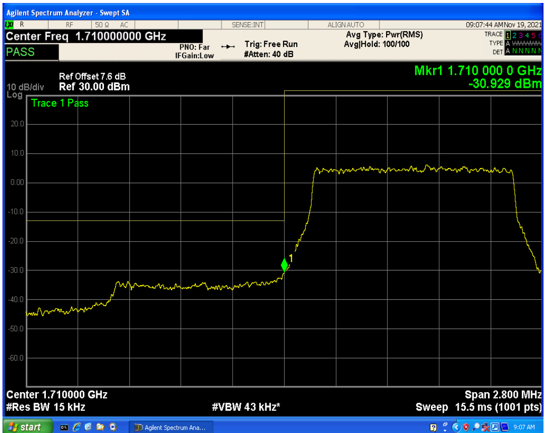
Band4 QPSK BW=10MHz Channel=20000 RB Size=1 Position=#Max
