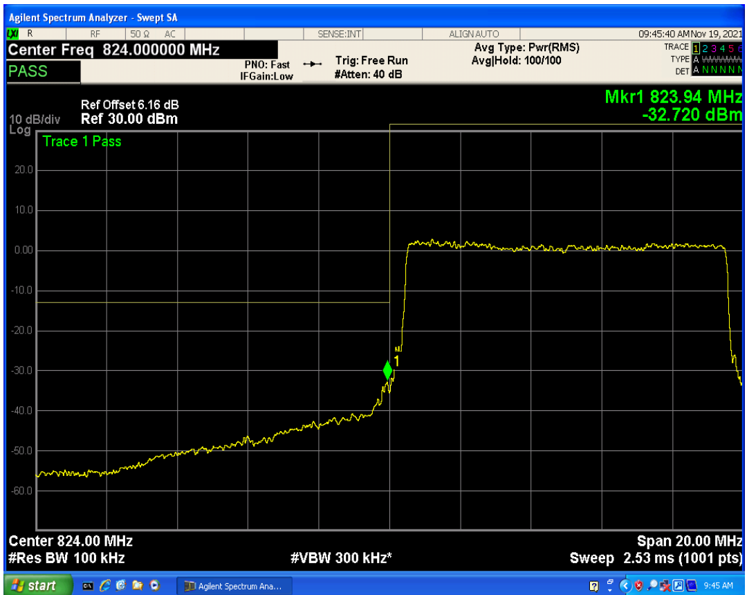
Band5 QAM16 BW=3MHz Channel=20415 RB Size=15 Position=#0
