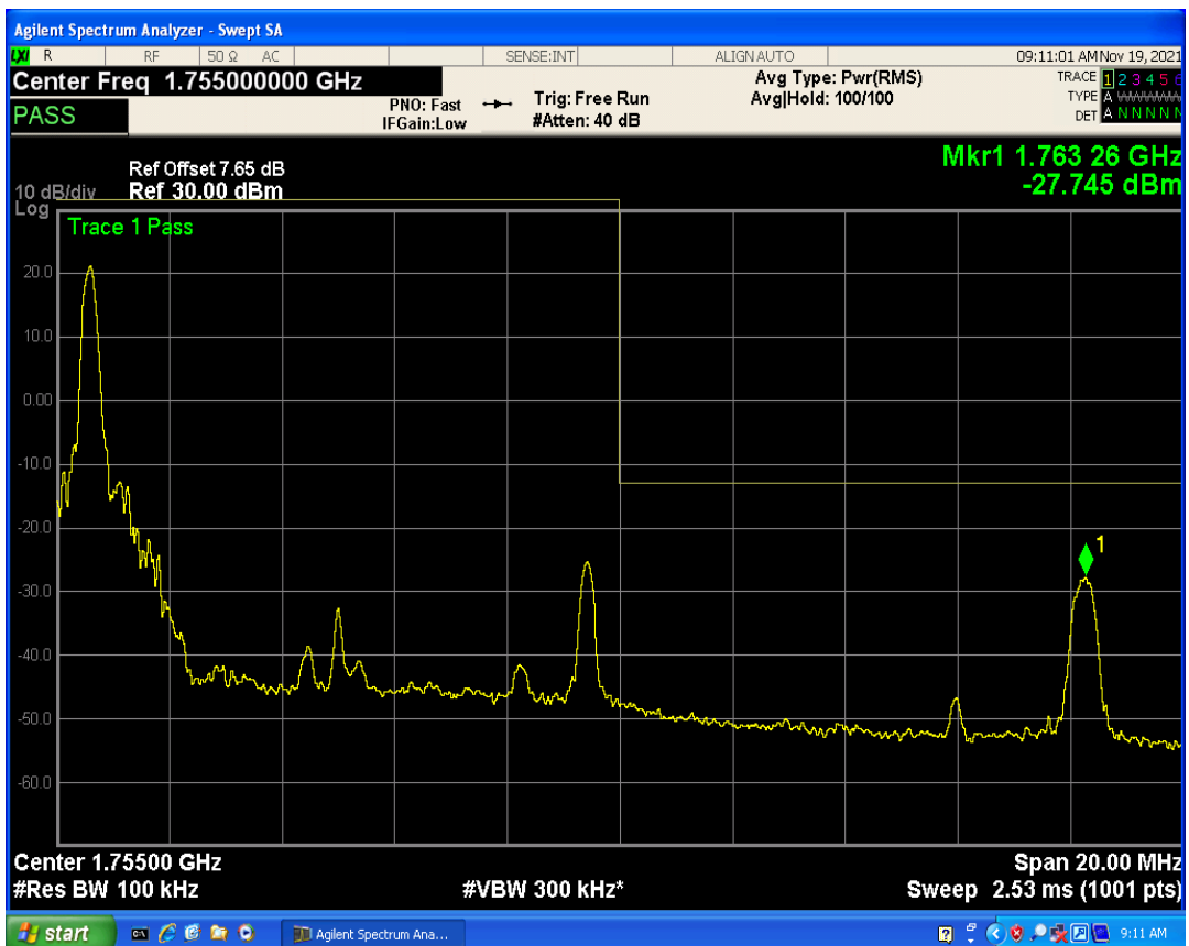
Band4 QAM16 BW=15MHz Channel=20325 RB Size=1 Position=#0
