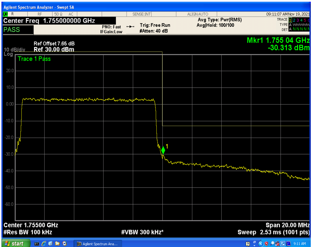
Band4 QAM16 BW=15MHz Channel=20025 RB Size=1 Position=#0
