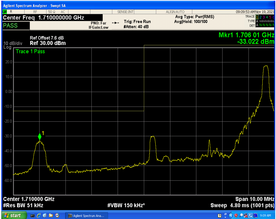
Band4 QPSK BW=1.4MHz Channel=19957 RB Size=1 Position=#0
