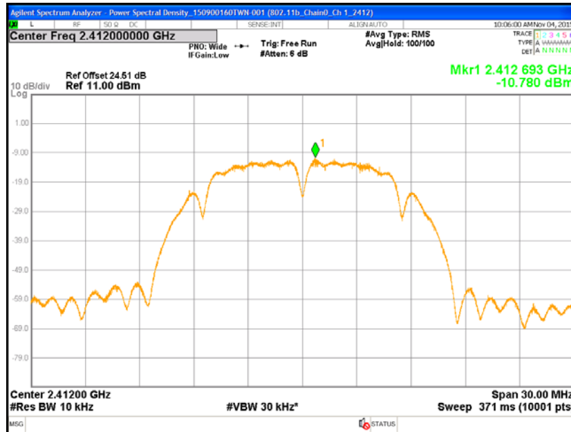
Chain0 : Power Spectral Density @ 802.11b mode Ch 1
