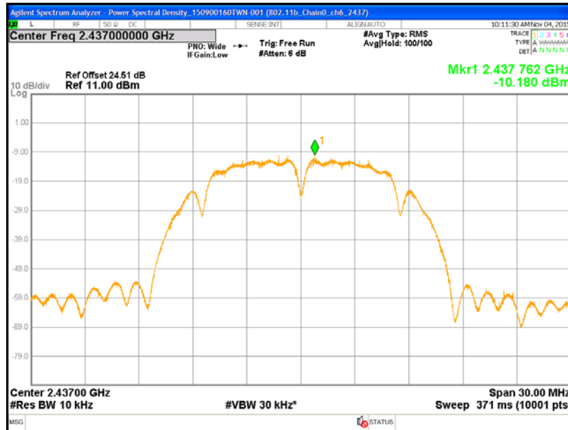
Chain0 : Power Spectral Density @ 802.11b mode ch6
