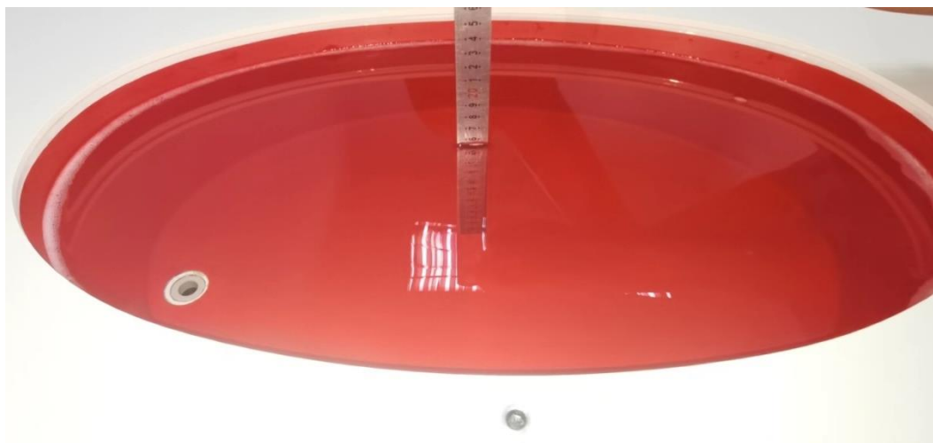
Picture 3: Liquid depth in the flat Phantom
