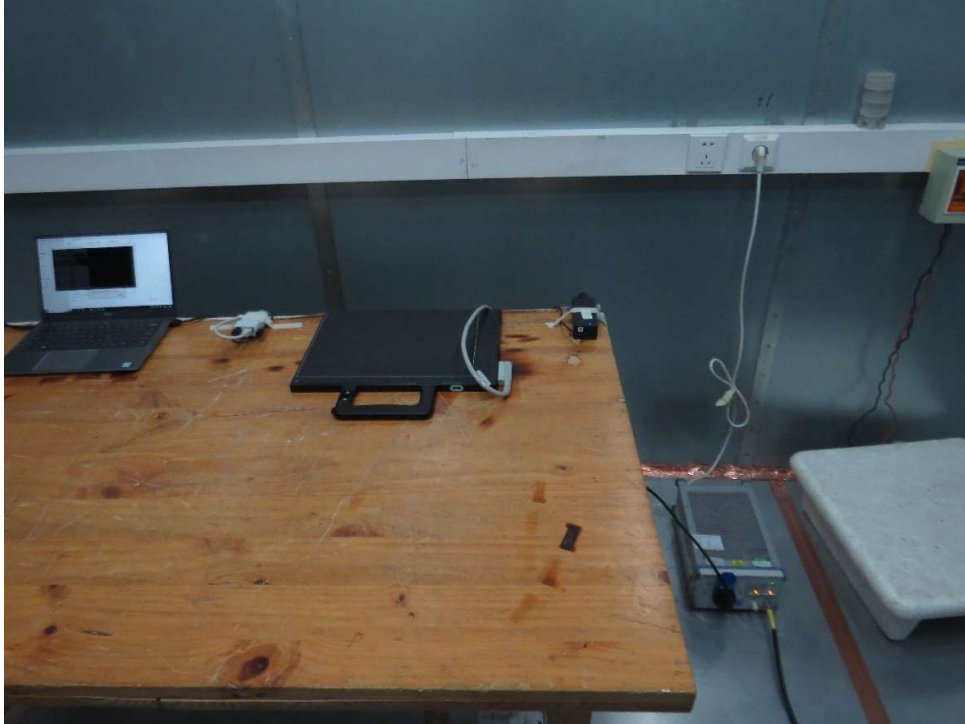
Picture 2 Conducted Emission Test Setup
