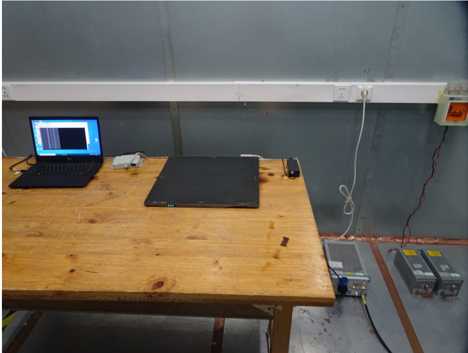
Picture 2 Conducted Emission Test Setup
