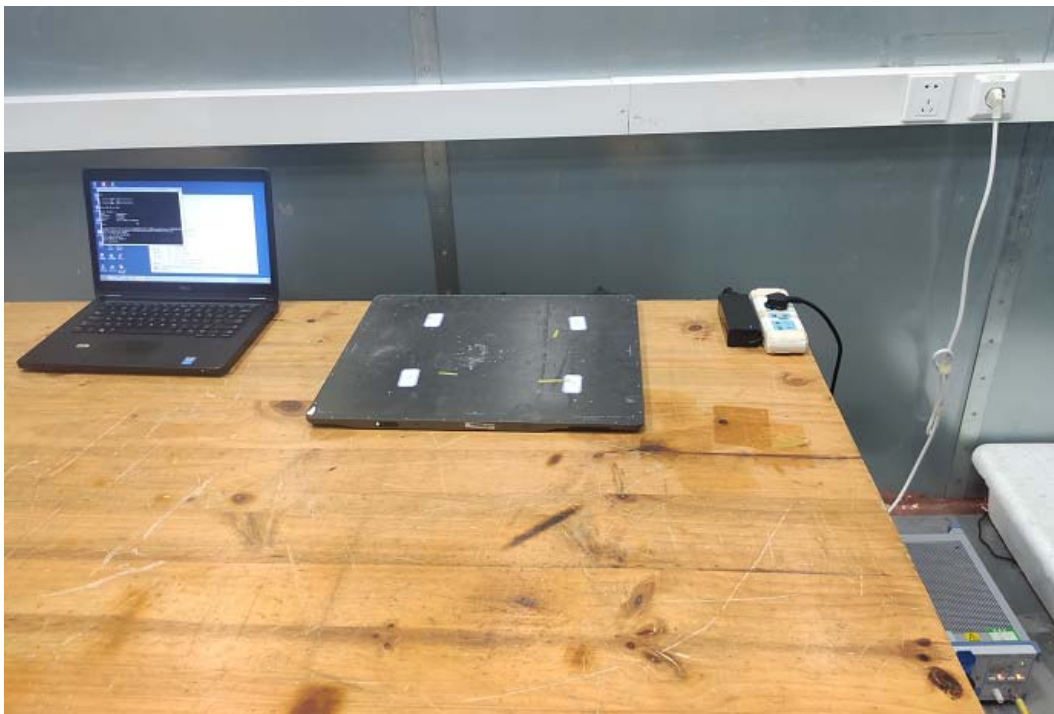
Picture 2 Conducted Emission Test Setup
