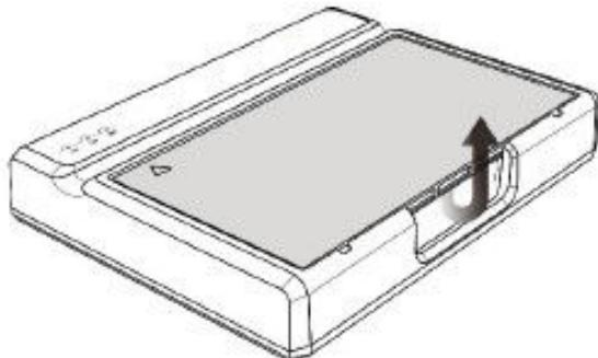
2. Insert battery into battery charger in the orientation shown below.
