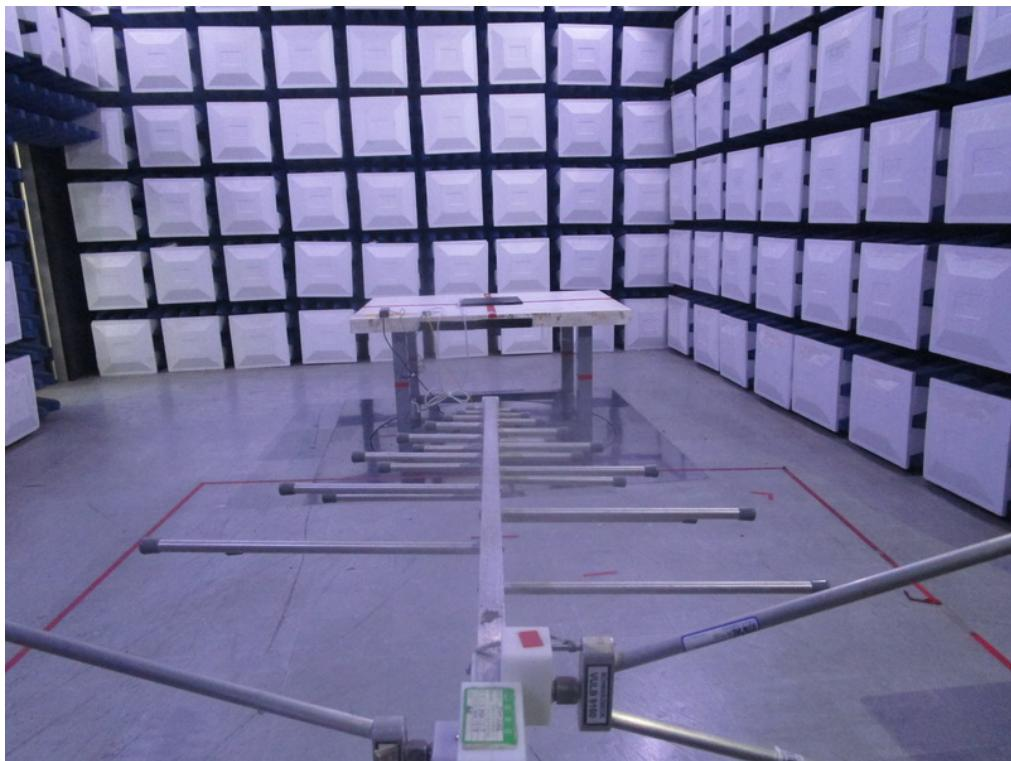
**Radiated Emissions Test Photos****Above 1 GHz**
