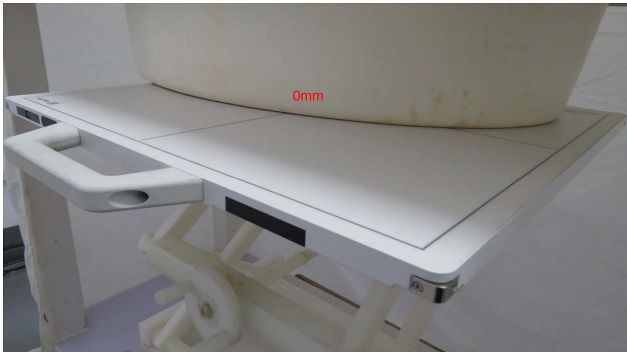
Picture 4: Front Side, the distance from handset to the bottom of the Phantom is 0mm (Scan 4)
