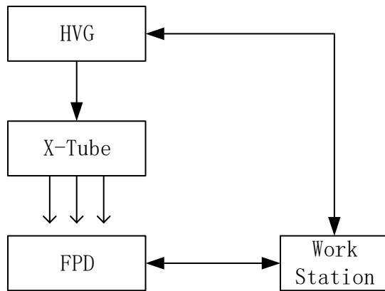
Workstation is a host device installed with iDetector and SDK. Chapter 3 has described how to establish connection between panels and workstation. In software mode, workstation does not control x-ray generator. Users would decide when to shoot x-ray.
