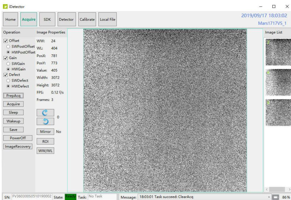
Status bar shows detector's serial number, the current task and state of detector, and feedback information of command. Status bar is also can be seen in other pages, and they are all same.
