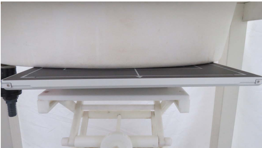
Picture 6: Front Side, the distance from handset to the bottom of the Phantom is 0mm (Scan 2)
