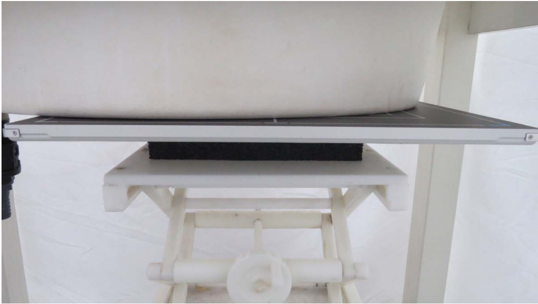
Picture 5: Front Side, the distance from handset to the bottom of the Phantom is 0mm (Scan 1)
