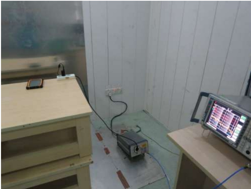
FCC RADIATED EMISSION TEST SETUP
