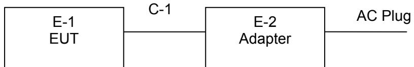
Radiated Spurious Emission Test
