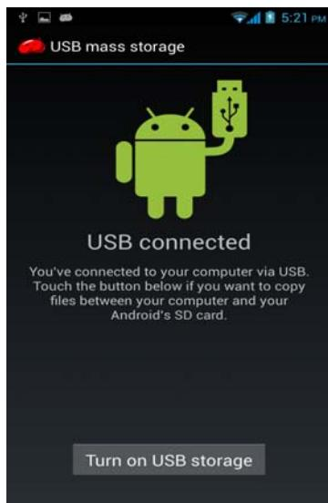
You can interact with the computer only by clicking to open the USB storage device, otherwise cannot interact, when you open a USB storage device, the icon will show off USB storage device, when you click again the mobile phone and the computer will stop interaction.
