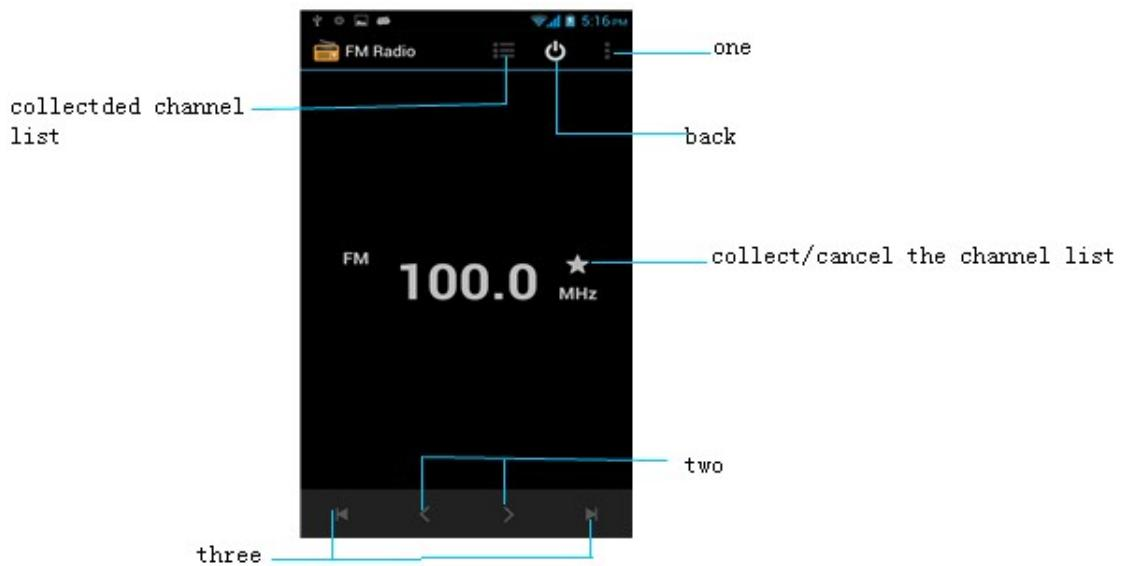
Tip: Need to wear headphones or install the antenna to receive.
