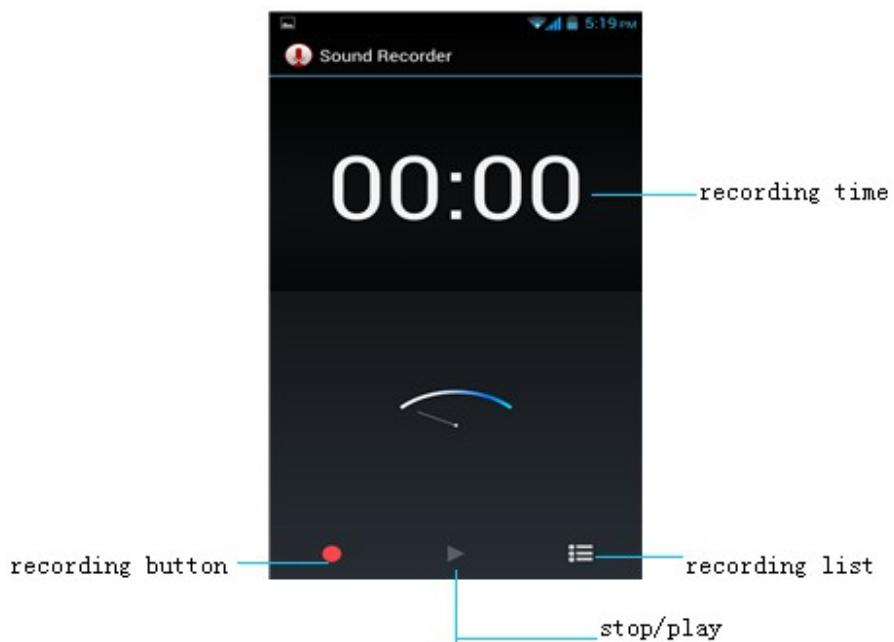
Press the menu button can also view the list of recordings and settings, including: can modify the type of recording file, whether to use high quality recordings and open sound.
