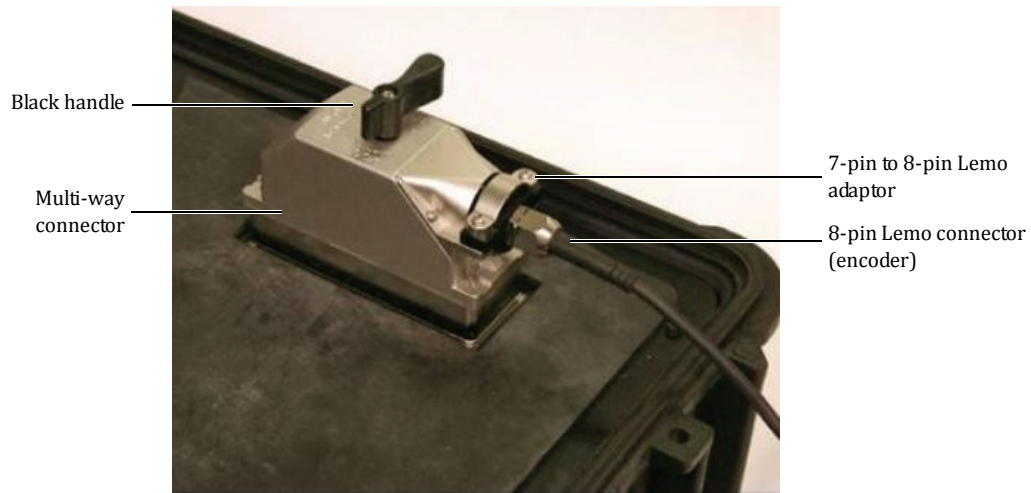
Figure 5-4 Connection to the RapidScan2
