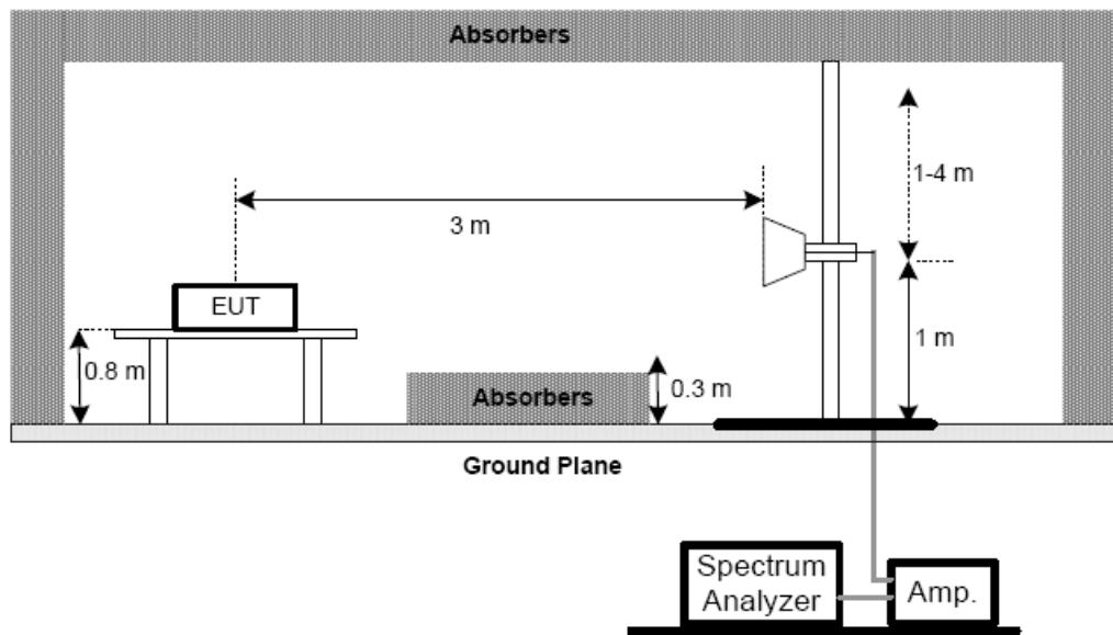
(C) For radiated emissions below 30MHz
