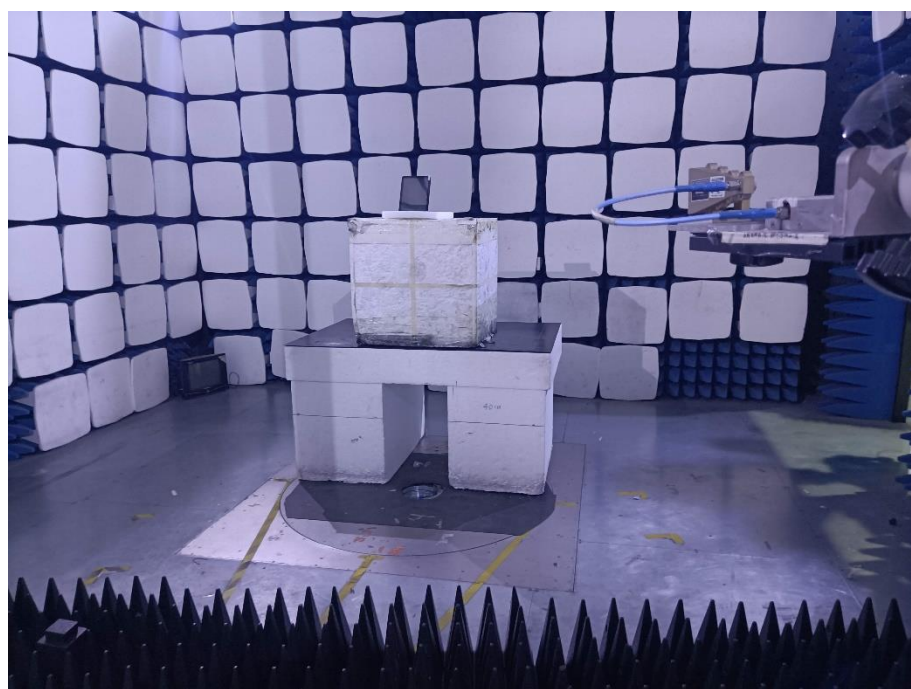
Radiation Emission Test Setup (Above18GHz)
