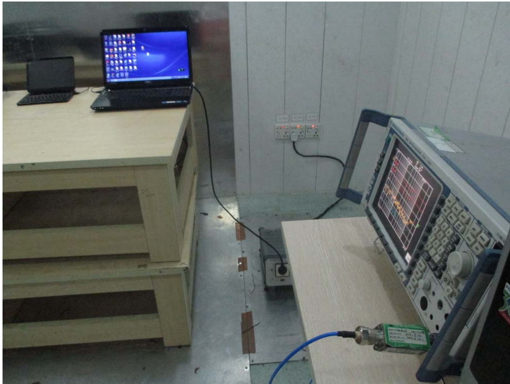
FCC RADIATED EMISSION TEST SETUP
