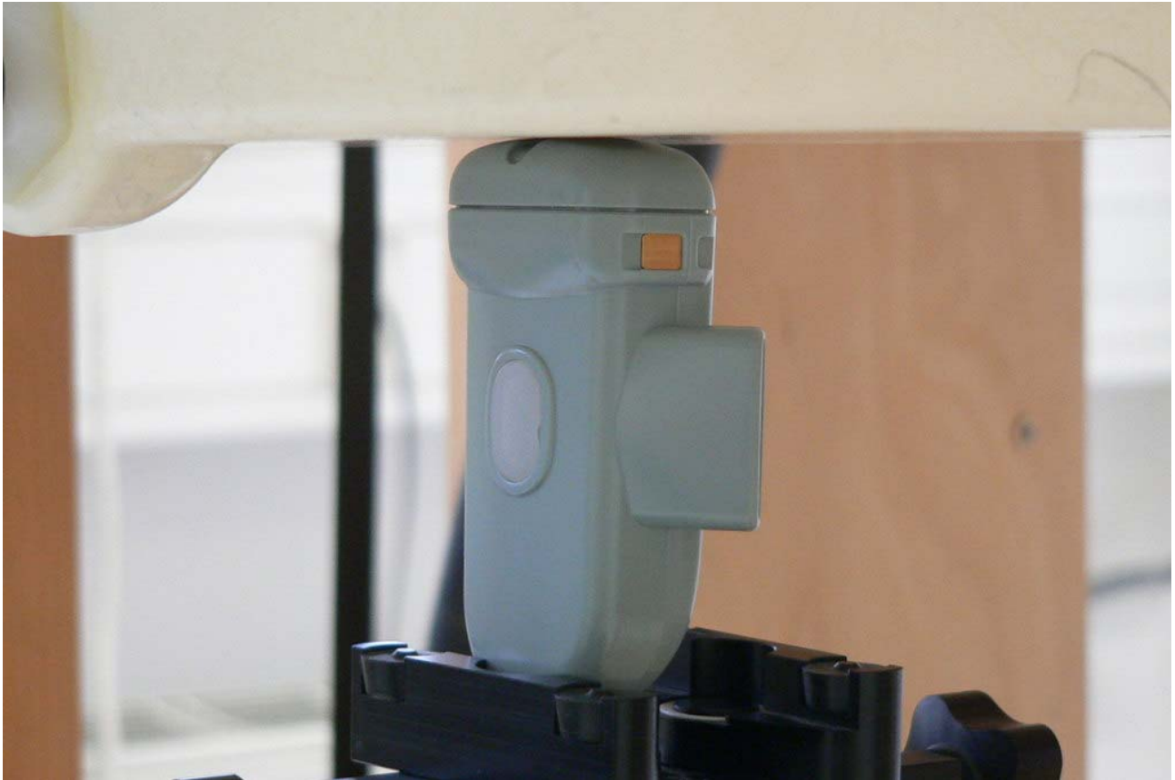
Fig. 12: Top side of OM247 SOLO2 3G 915MHz towards the phantom, 0 mm distance.
