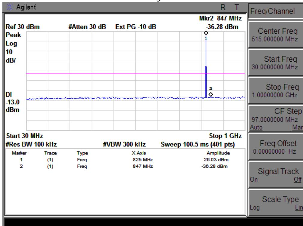
Conducted Emission Transmitting Mode CH 128 1MHz – 10GHz
