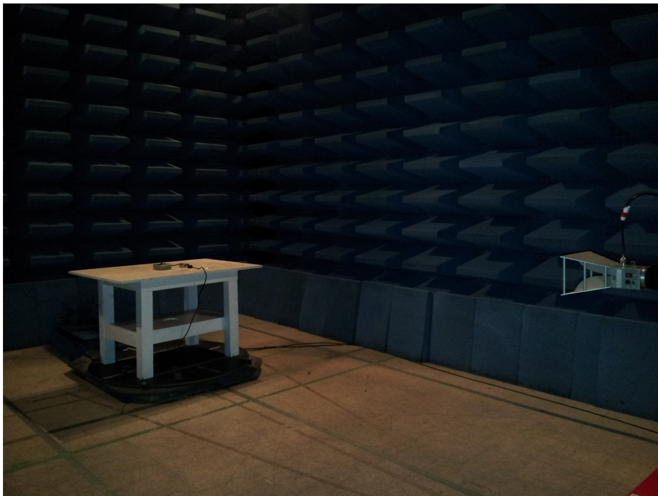
Figure 31: Emissions Test Setup – Intentional Harmonics(1-10GHz)
