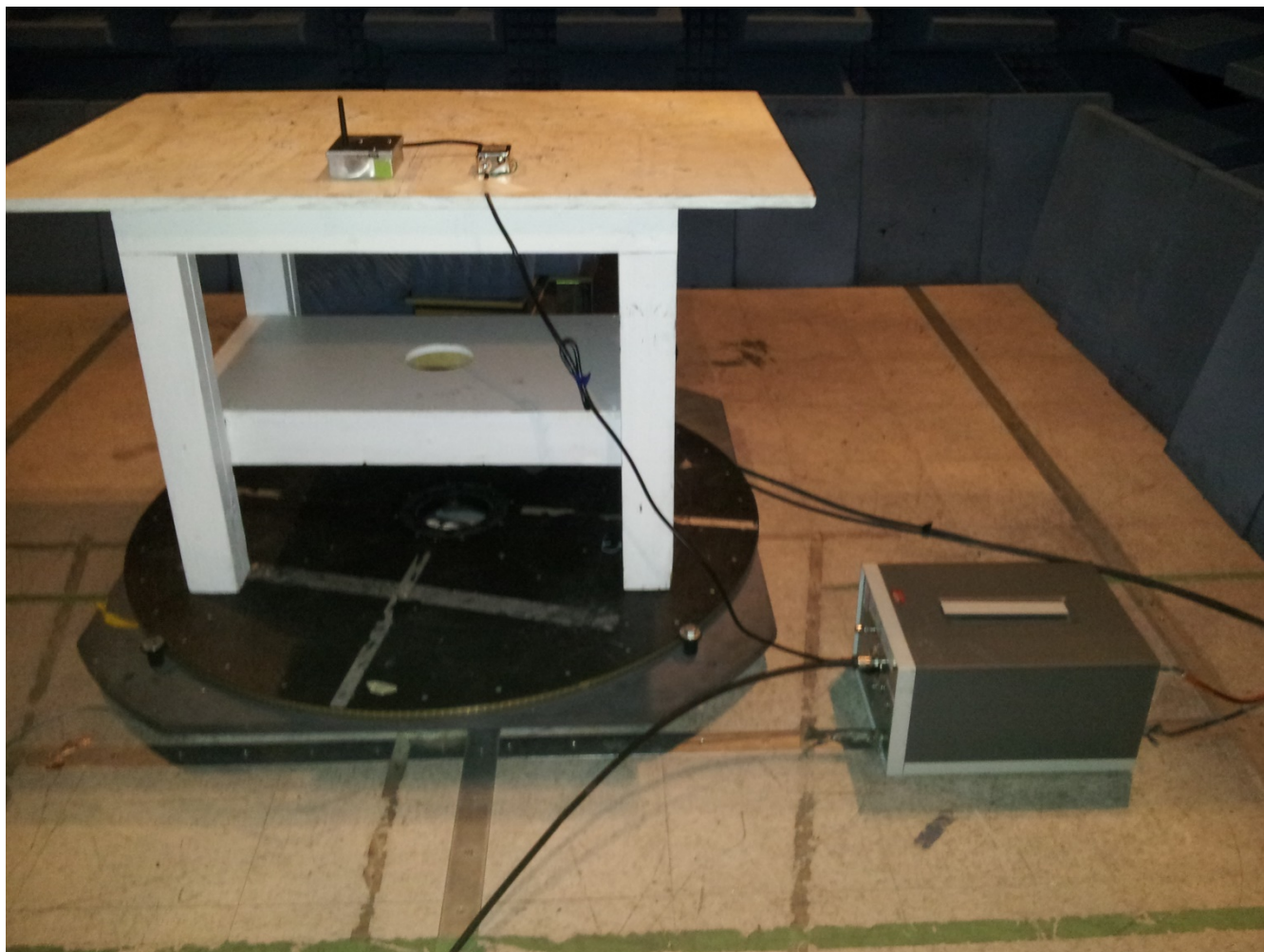
Figure 29:Emissions Test Setup – AC Mains Conducted Emissions
