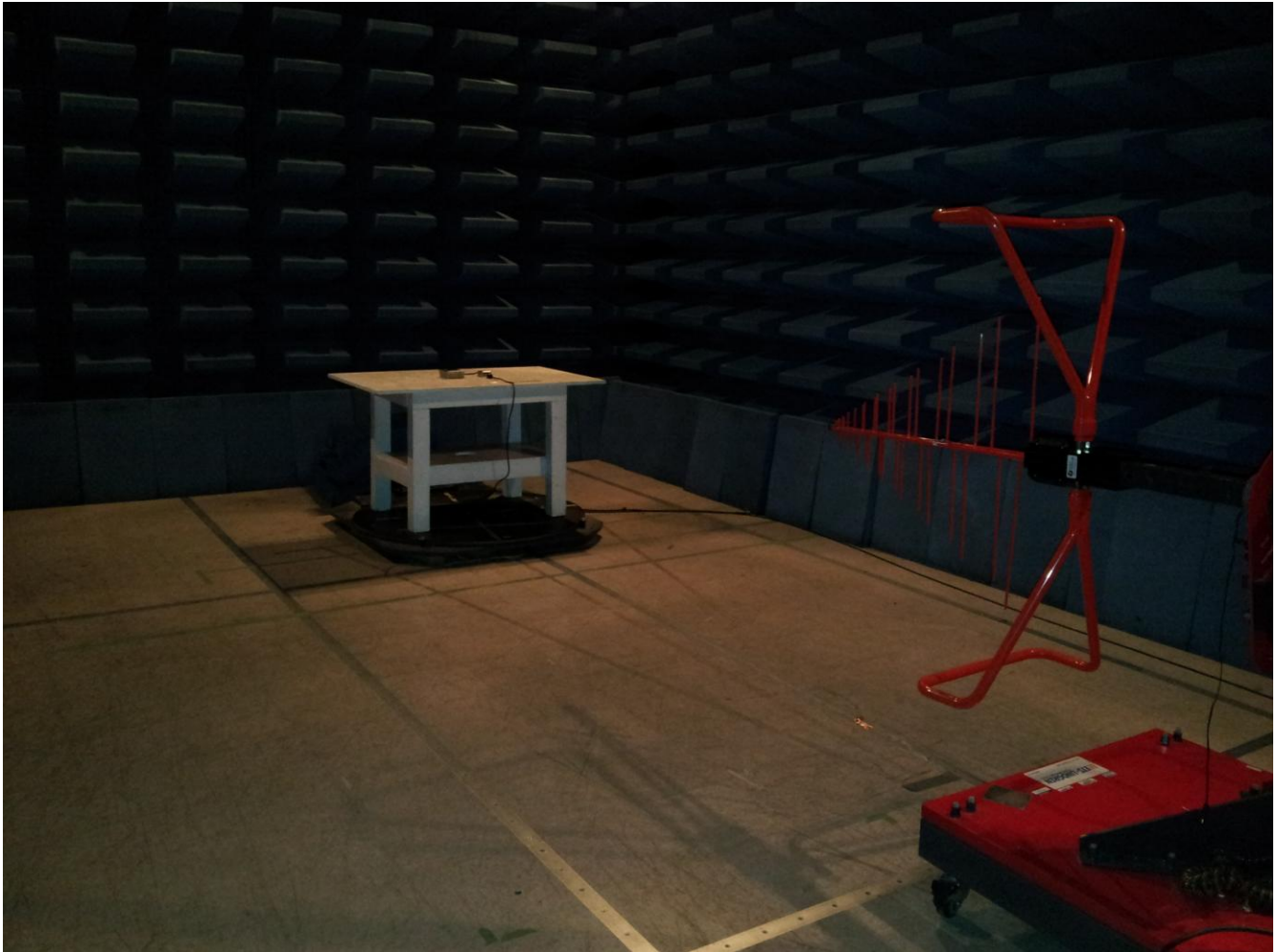
Radiated Emissions Test Setup – Intentional / Unintentional Radiated Emissions
