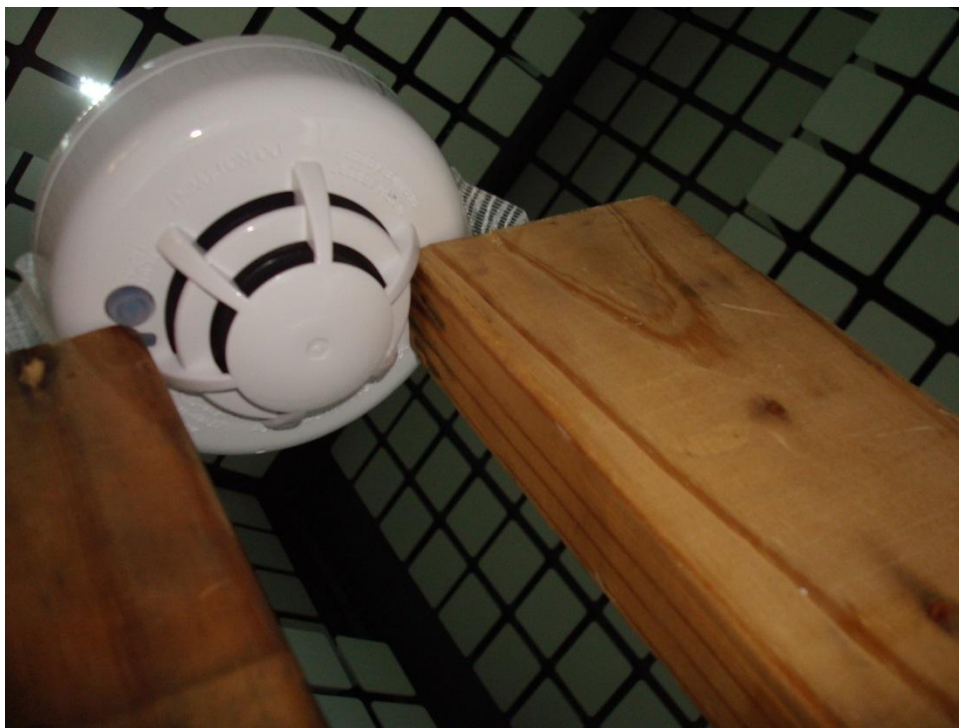
Figure 8 - Radiated Emissions Test Setup
