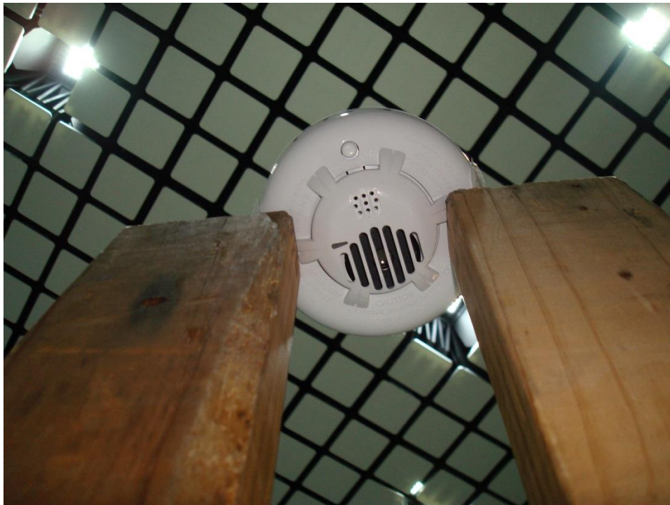
Figure 8 - Radiated Emissions Test Setup
