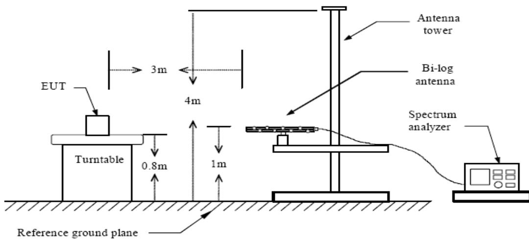
For radiated spurious emissions above 1GHz
