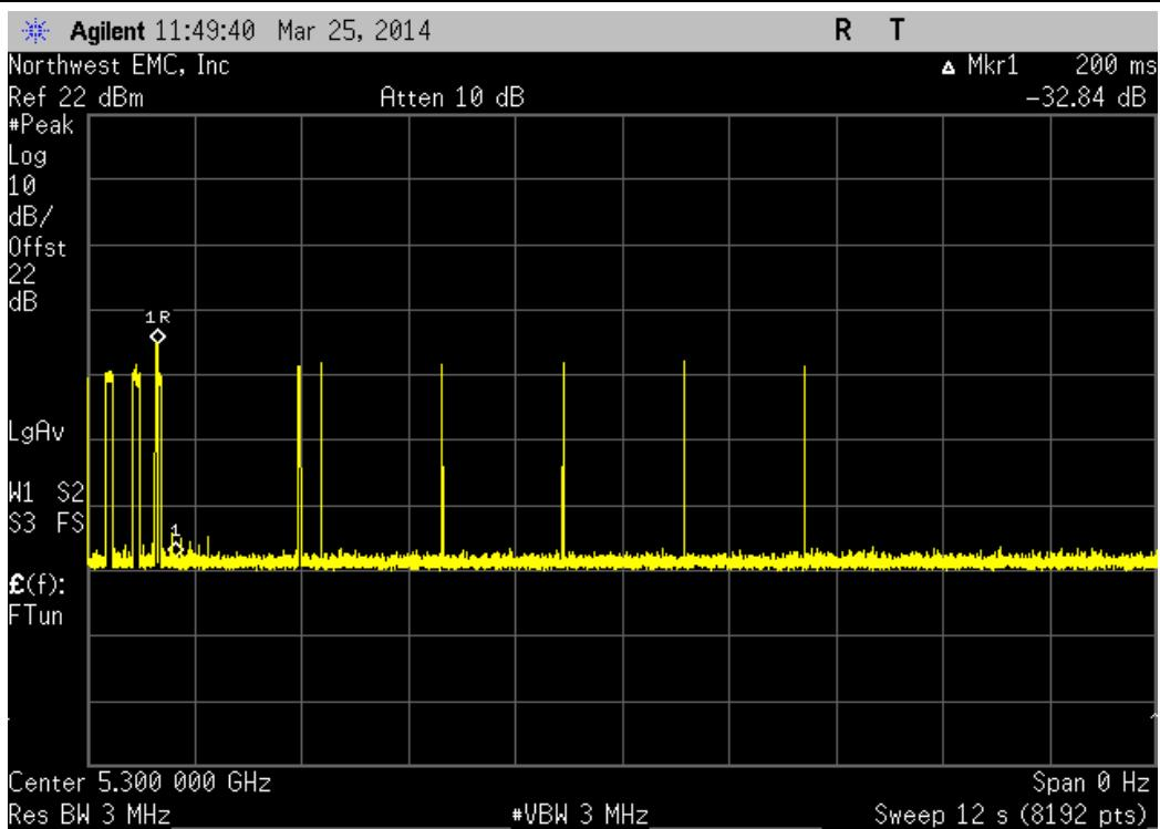
20MHz, 5560 MHz, Radar 1 Control Signal Pulse Width
