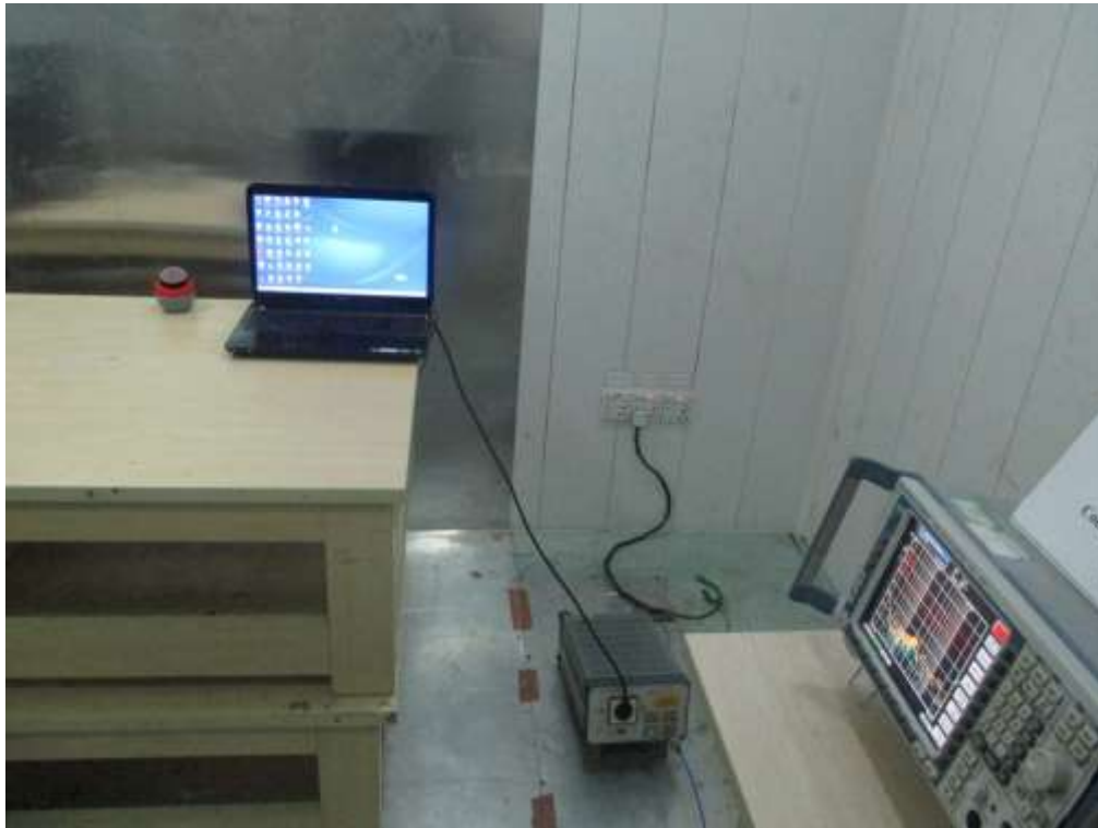
FCC RADIATED EMISSION TEST SETUP
