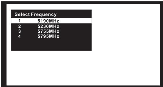
Step 2: Press the frequency adjusting button again to choose the desired frequency range. After 3 seconds, the system will save the selected frequency automatically.
