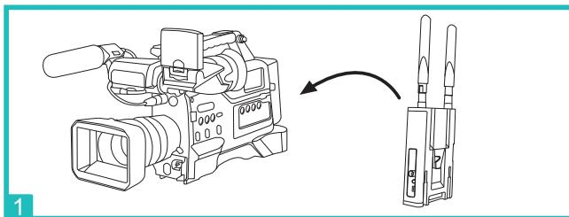
Install V-Mount battery of camera into battery mount of transmitter or use the external power adaptor instead of the battery
