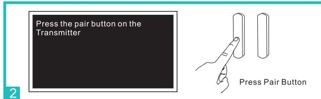
**Step3:** Press the Pair button on the transmitter
