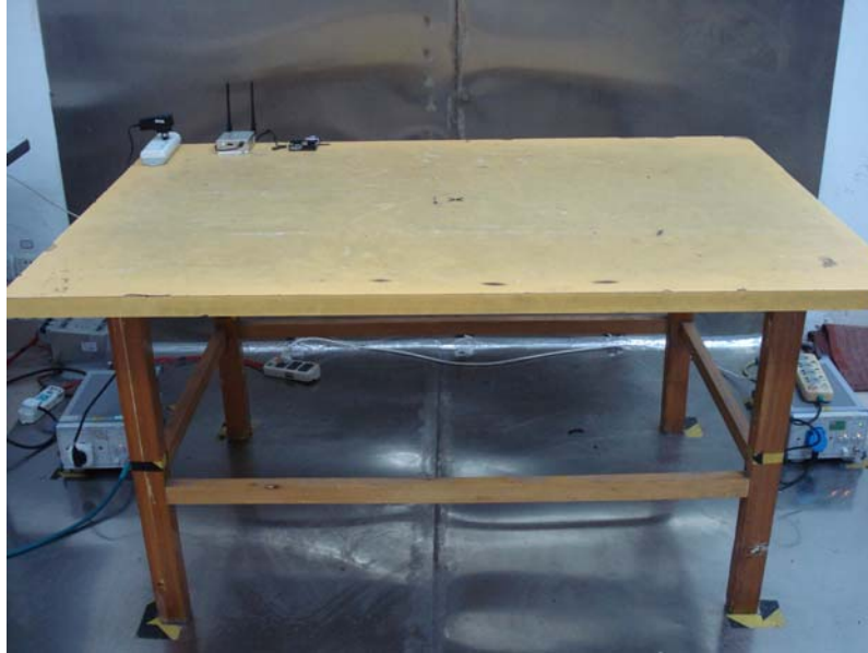
Conducted Emissions Test Setup – Front View
