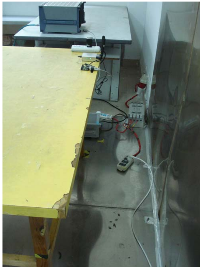
Conducted Emissions Test Setup – Side View
