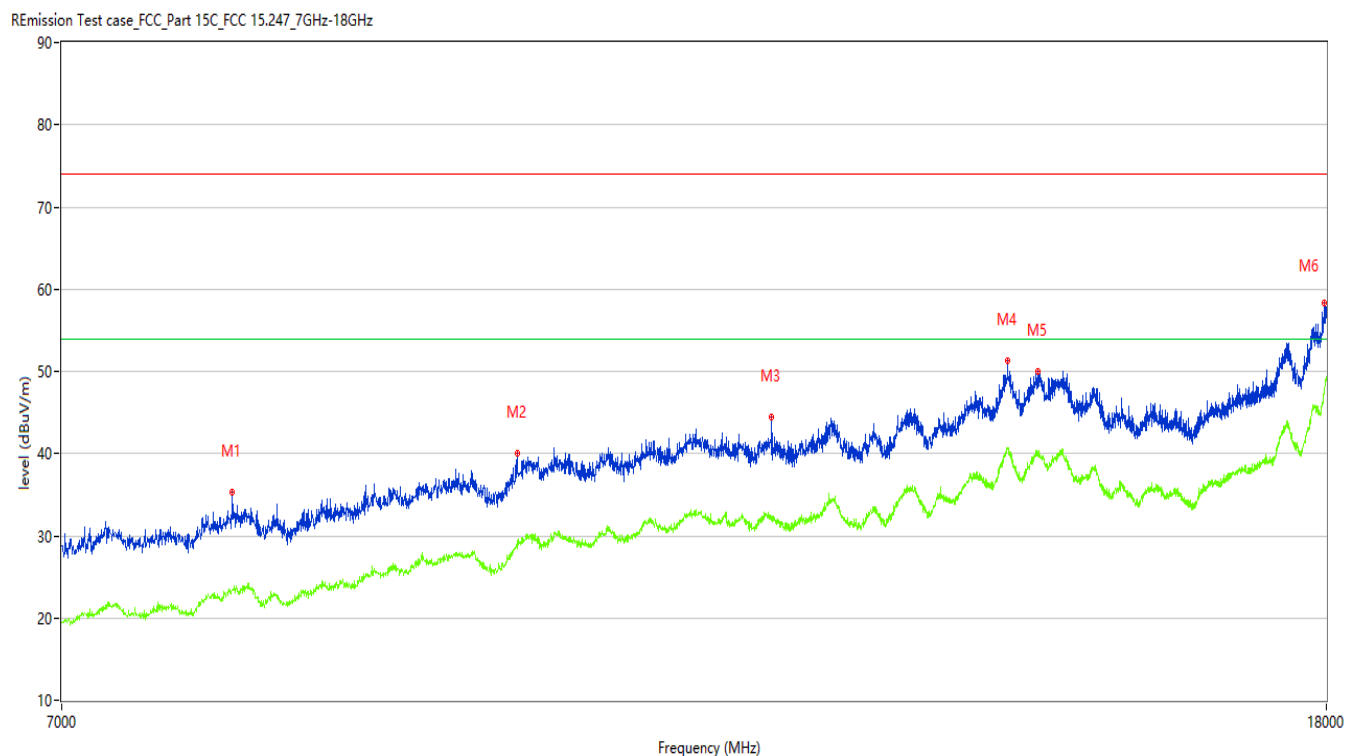
Figure 31: Radiated Emission, BLE-1M, 2480MHz_7GHz_18GHz Horizontal polarization
