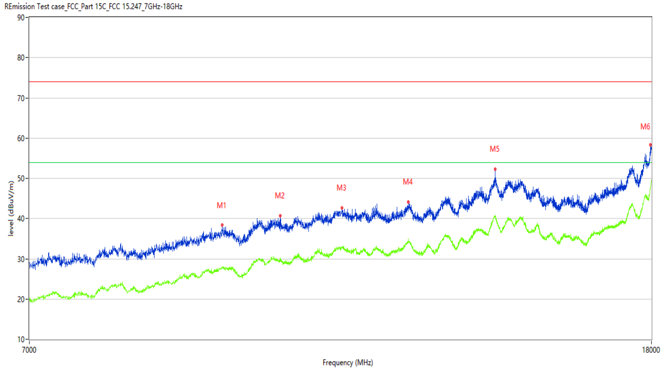
Figure 29: Radiated Emission, BLE-1M, 2440MHz_7GHz_18GHz Horizontal polarization
