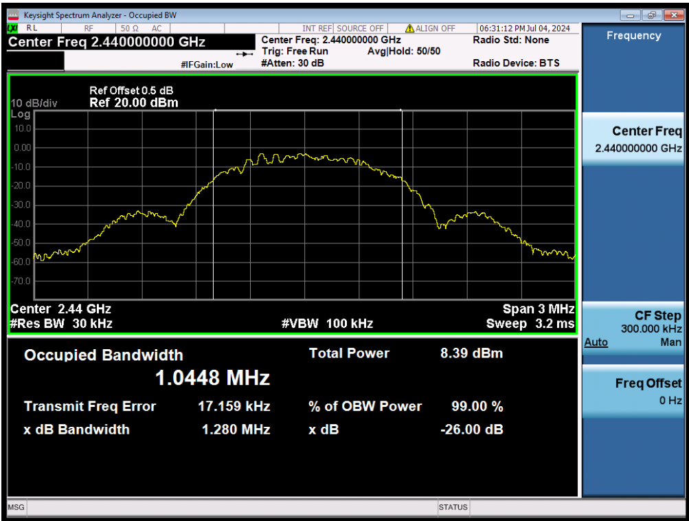
99% Bandwidth, 2440MHz, BLE-1Mbps
