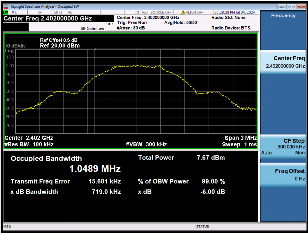
99% Bandwidth, 2402MHz, BLE-1Mbps
