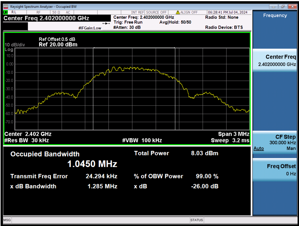
99% Bandwidth, 2402MHz, BLE-1Mbps
