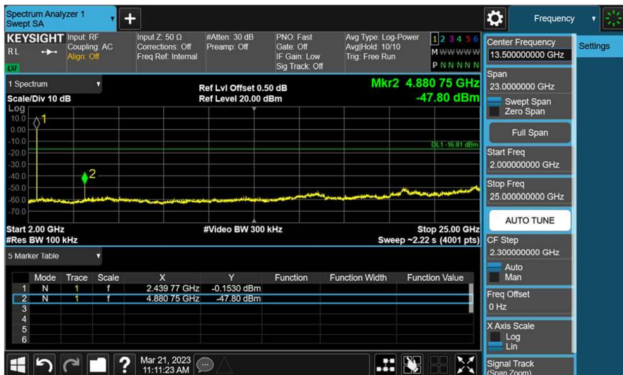
Figure 45: Conducted Spurious Emission & Authorized-band band-edge, 2480MHz, BLE-1M Carrier Level
