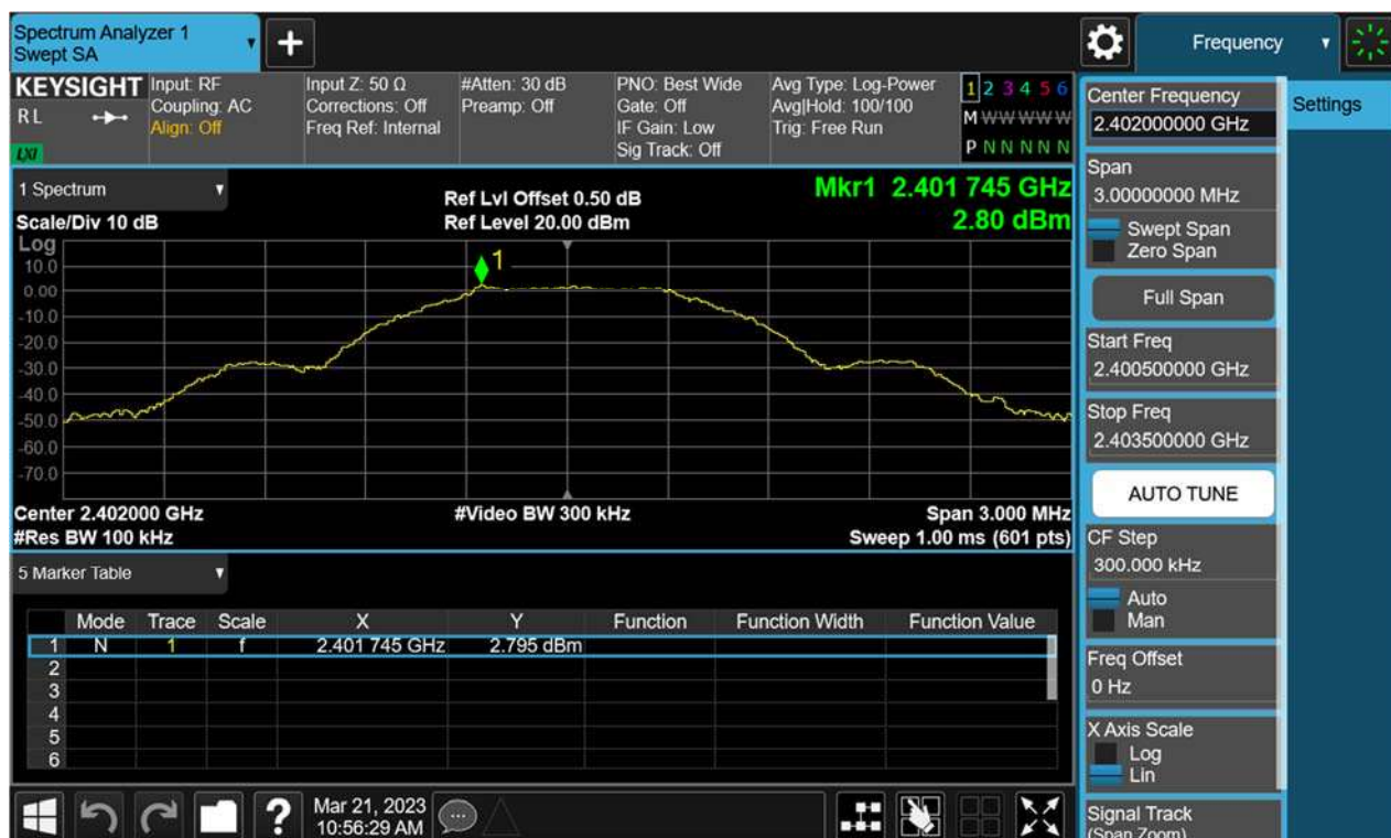
Figure 43: Conducted Spurious Emission & Authorized-band band-edge, 2402MHz, BLE-1M Carrier Level
