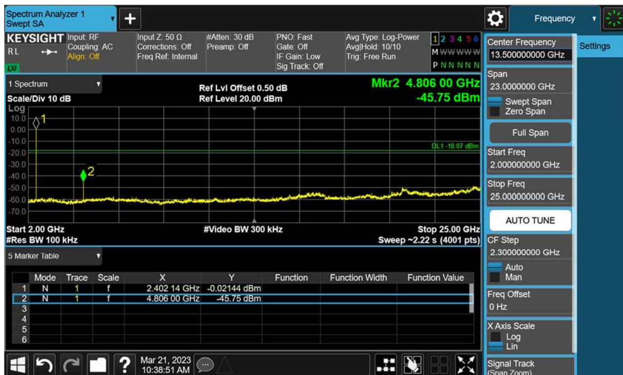
Figure 41: Conducted Spurious Emission & Authorized-band band-edge, 2440MHz, BLE-2M Carrier Level
