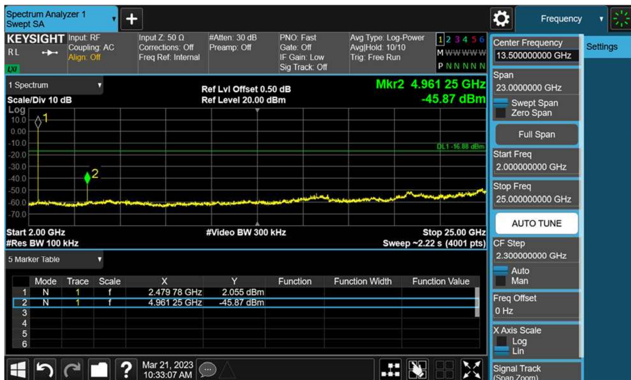
Figure 40 Conducted Spurious Emission & Authorized-band band-edge, 2402MHz, BLE-2M Carrier Level
