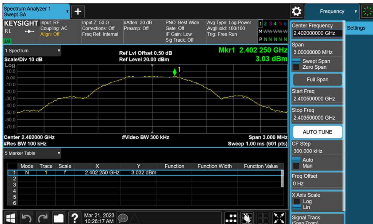
Figure 37: Conducted Spurious Emission & Authorized-band band-edge, 2402MHz, BLE-1M Carrier Level
