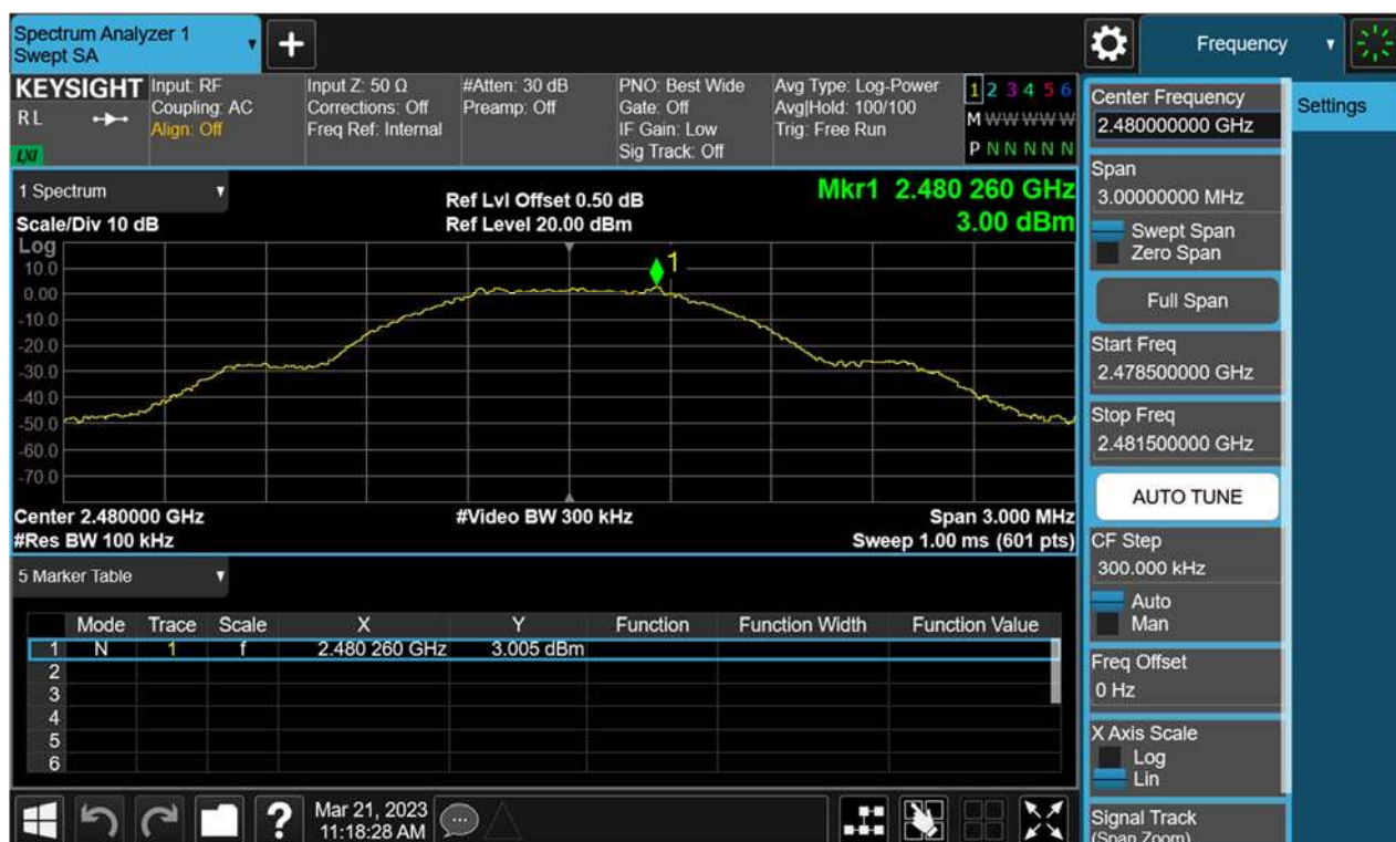
Figure 45: Conducted Spurious Emission & Authorized-band band-edge, 2480MHz, BLE-1M Carrier Level
