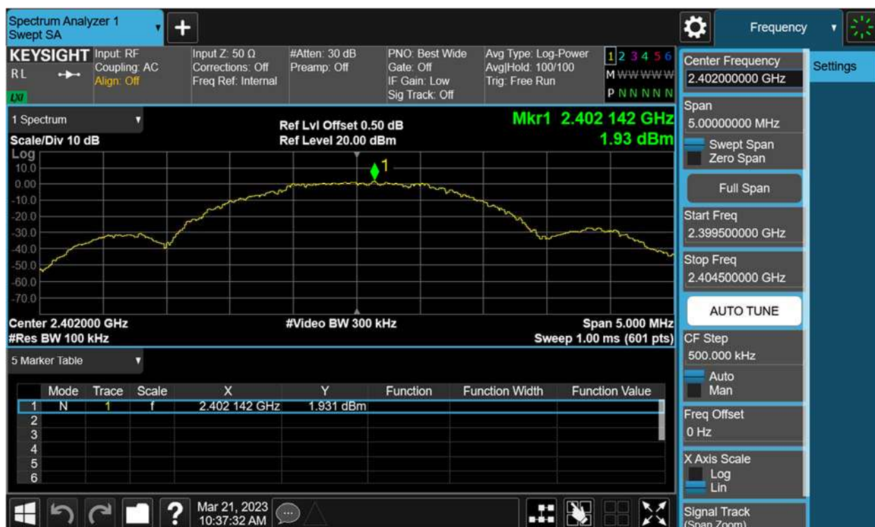
Figure 40 Conducted Spurious Emission & Authorized-band band-edge, 2402MHz, BLE-2M Carrier Level
