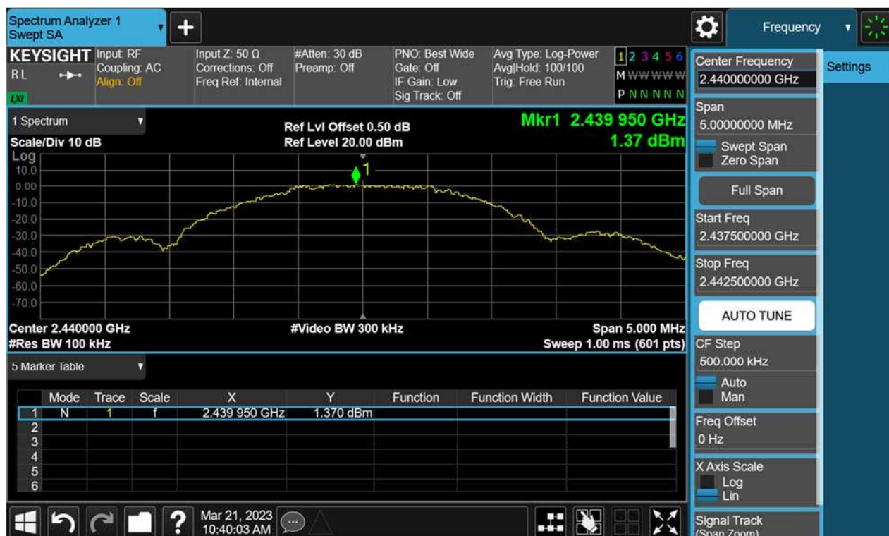
Figure 41: Conducted Spurious Emission & Authorized-band band-edge, 2440MHz, BLE-2M Carrier Level
