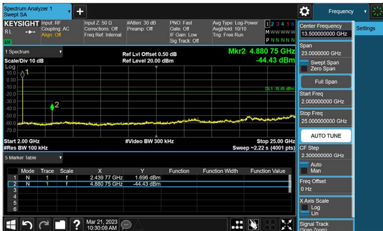
Figure 39: Conducted Spurious Emission & Authorized-band band-edge, 2480MHz, BLE-1M Carrier Level
