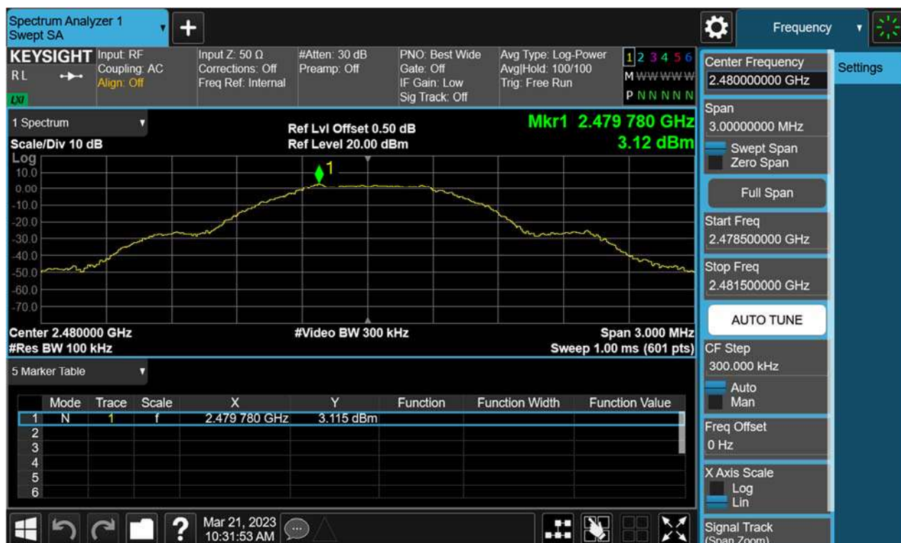
Figure 39: Conducted Spurious Emission & Authorized-band band-edge, 2480MHz, BLE-1M Carrier Level
