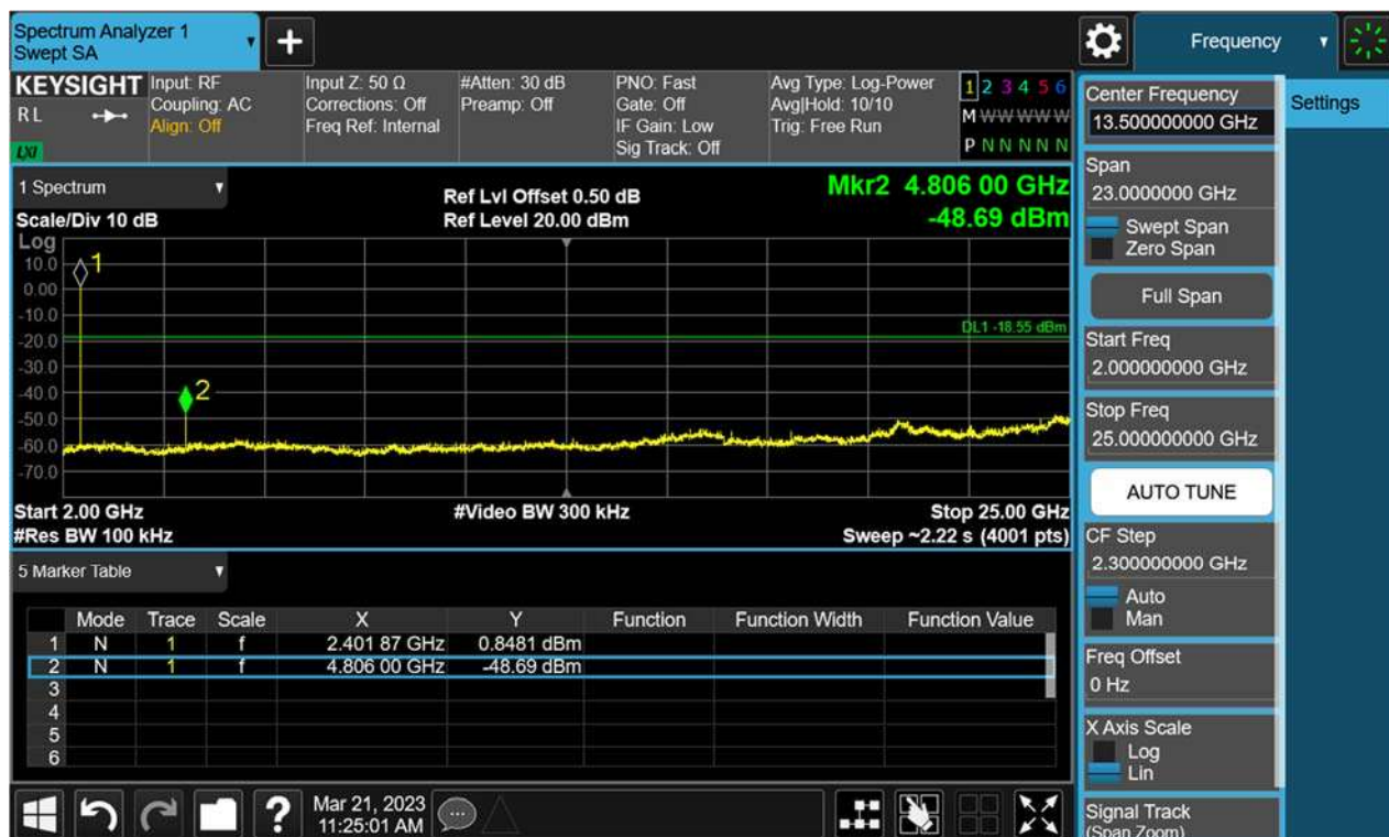
Figure 47: Conducted Spurious Emission & Authorized-band band-edge, 2440MHz, BLE-2M Carrier Level
