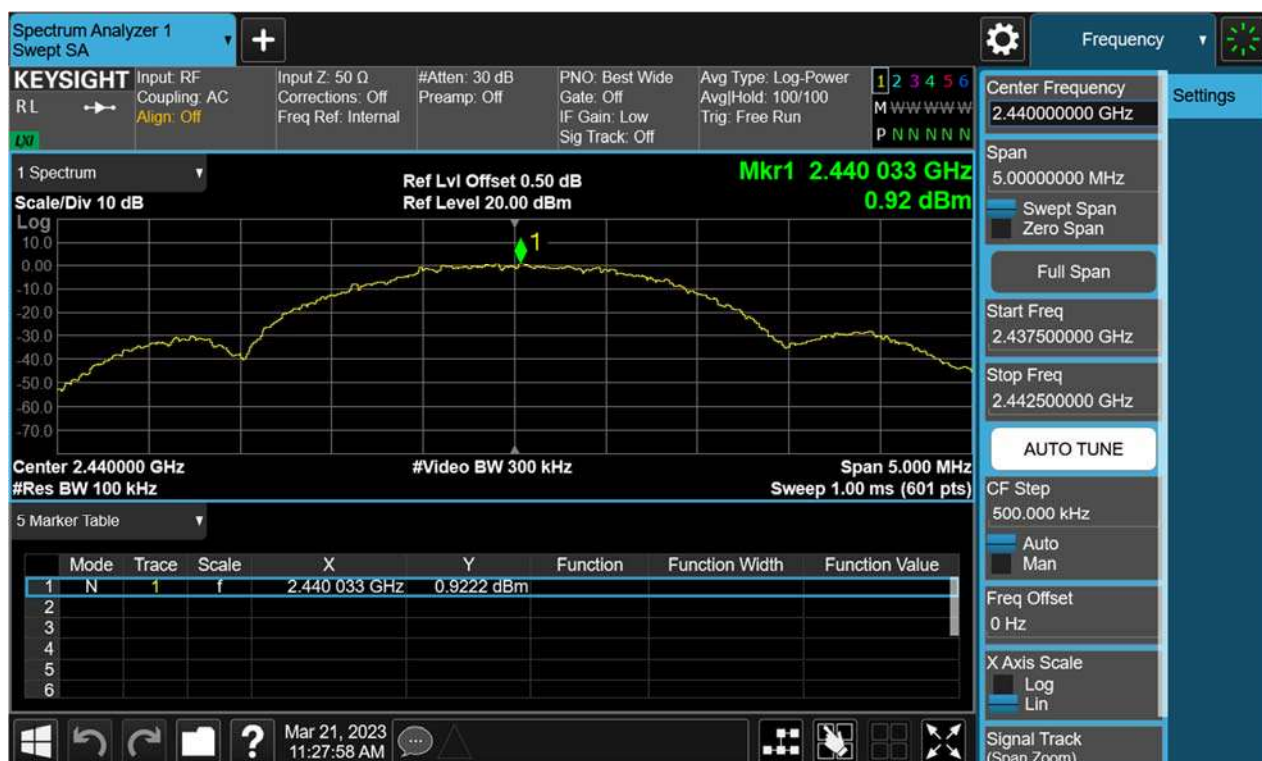
Figure 47: Conducted Spurious Emission & Authorized-band band-edge, 2440MHz, BLE-2M Carrier Level
