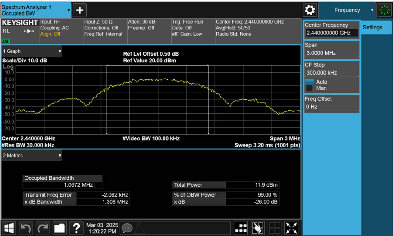
99% Bandwidth, 2440MHz, BLE-1Mbps
