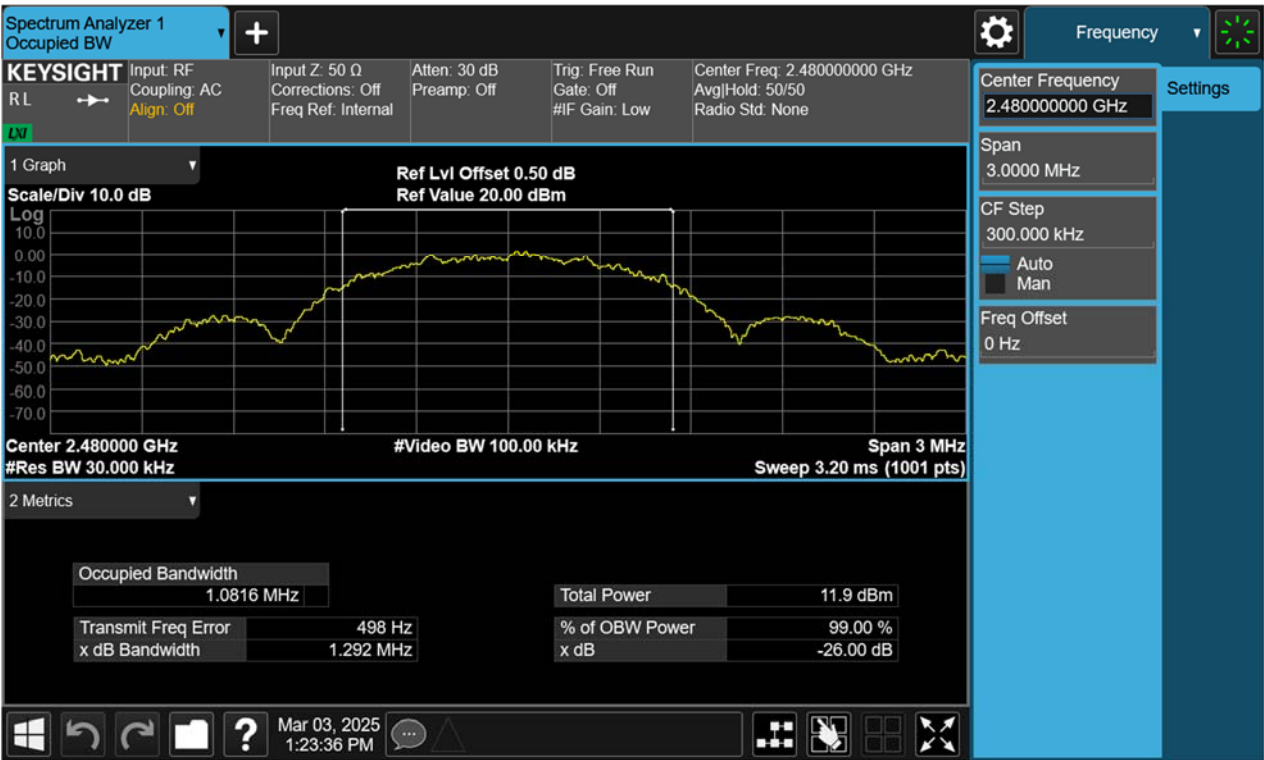
99% Bandwidth, 2480MHz, BLE-1Mbps
