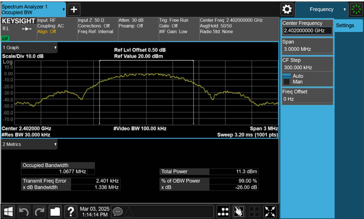
99% Bandwidth, 2402MHz, BLE-1Mbps
