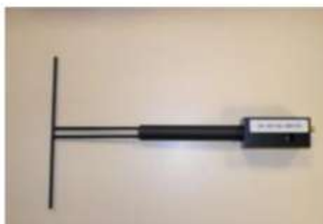
Figure 1 – Satimo COMOSAR Validation Dipole
