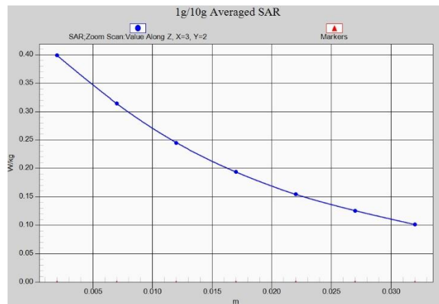
Fig. 1-1 Z-Scan at power reference point (GSM850)
