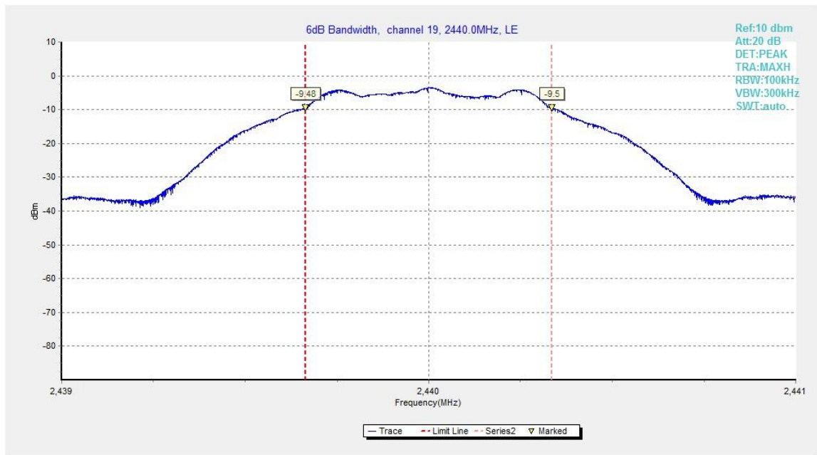
Fig.21. 6dB Bandwidth: GFSK, 2440 MHz
