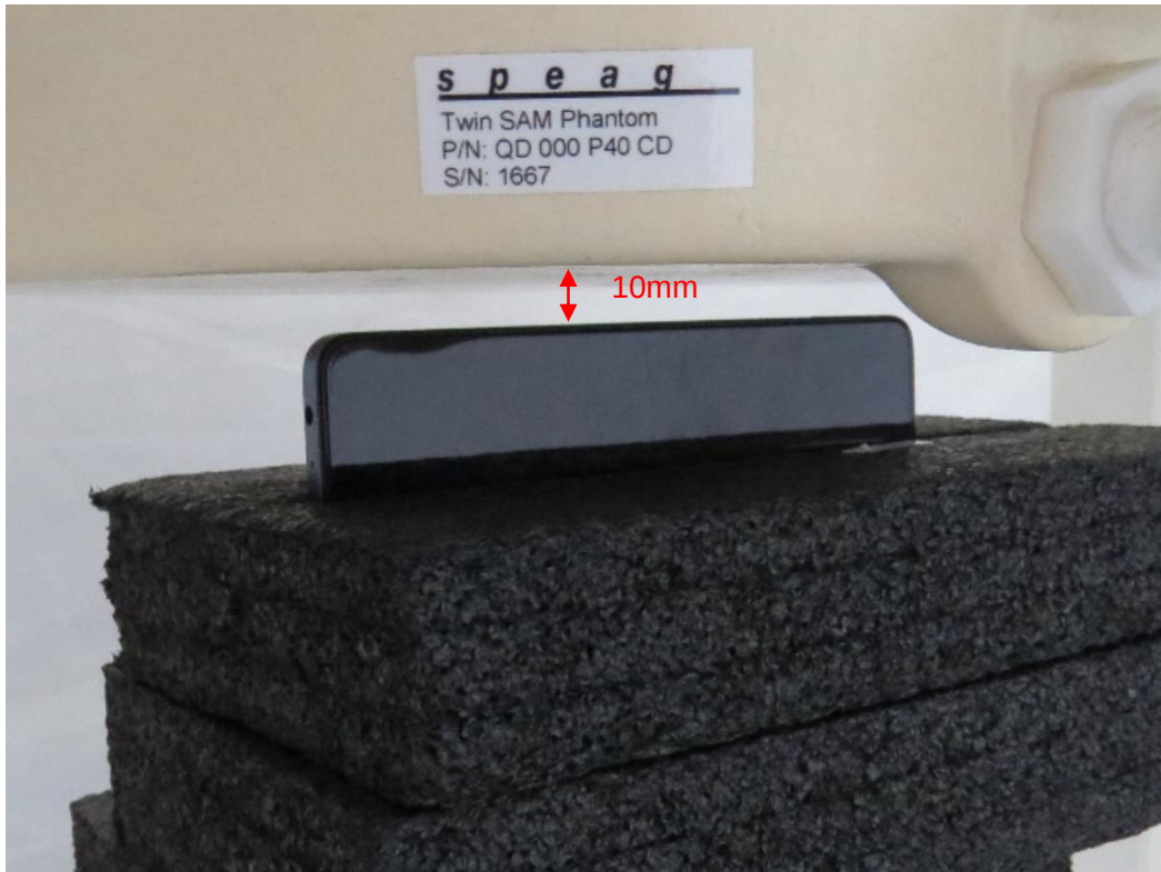
Picture 10: Left Edge, the distance from EUT to the bottom of the Phantom is 10mm
