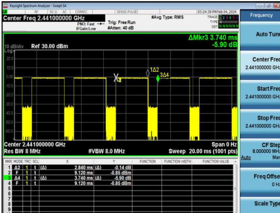
Note: Duty factor= Ton (ms)/ T(on+off) (ms)=2.840/3.740\*100%=75.9%
