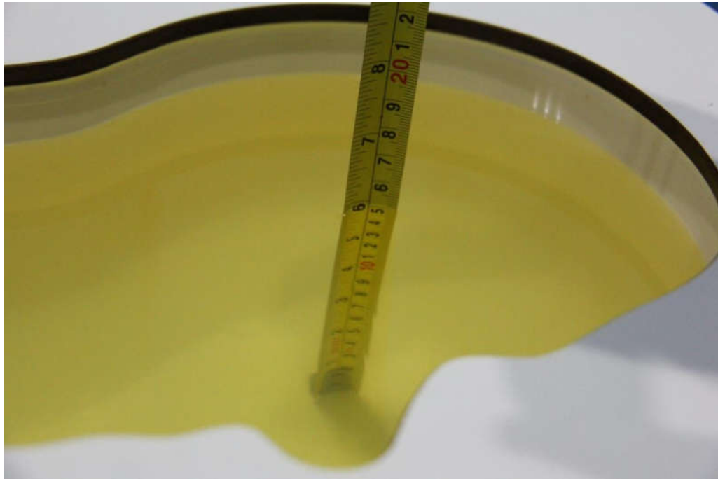
Picture 7-7: Liquid depth in the Head Phantom (3500MHz)
