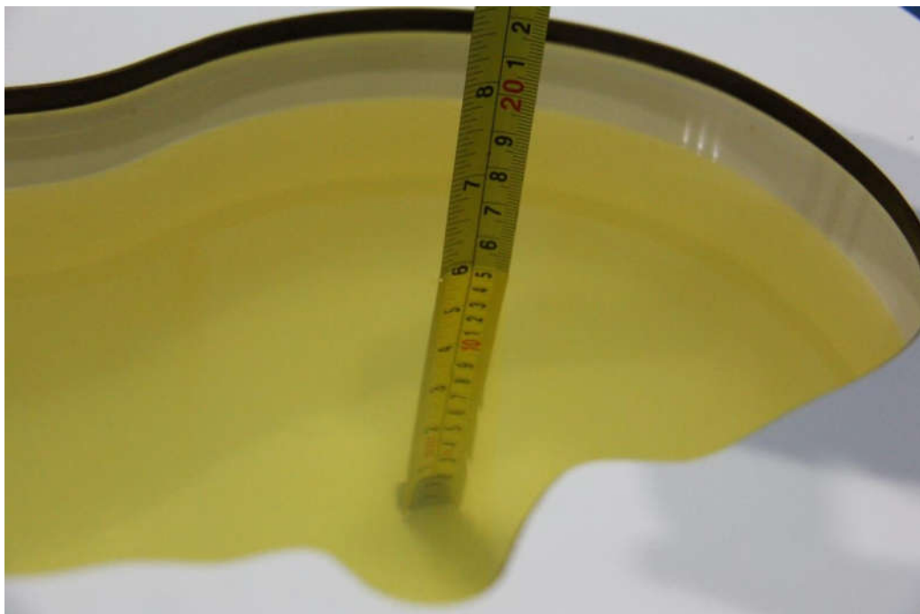
Picture 7-8: Liquid depth in the Head Phantom (3900MHz)
