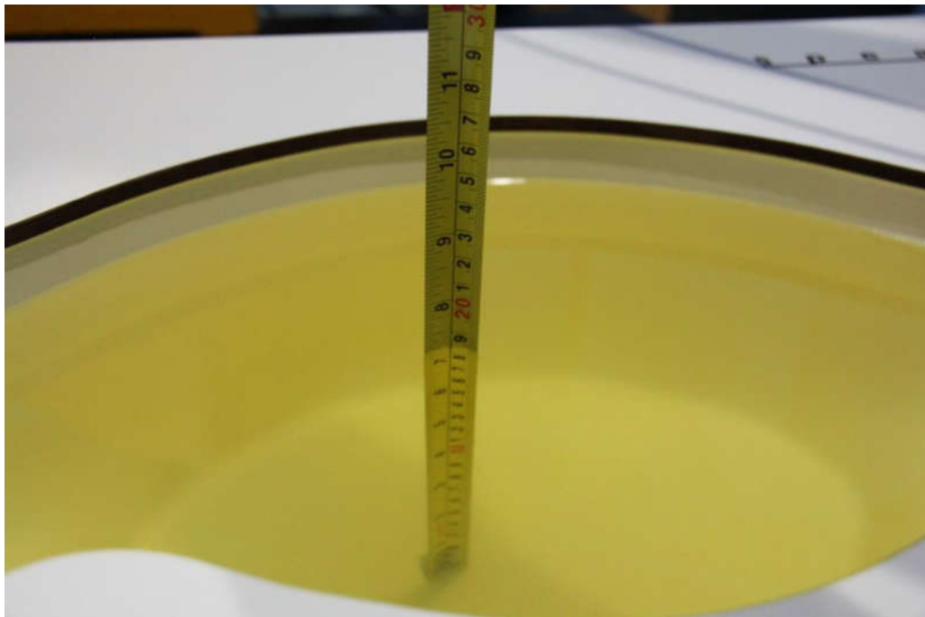
Picture 7-6: Liquid depth in the Flat Phantom (2550MHz)
