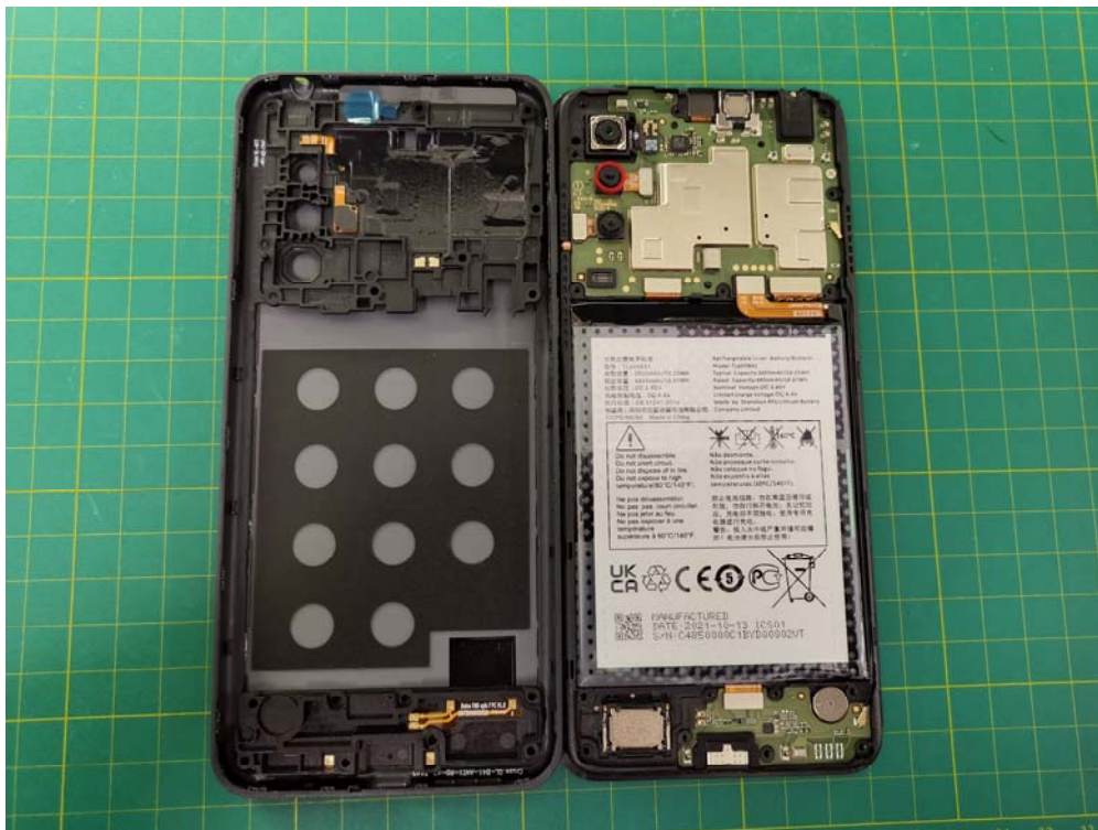
6102H Mobile Phone Disassembly
