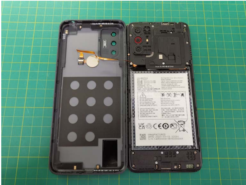
6102H Mobile Phone Disassembly
