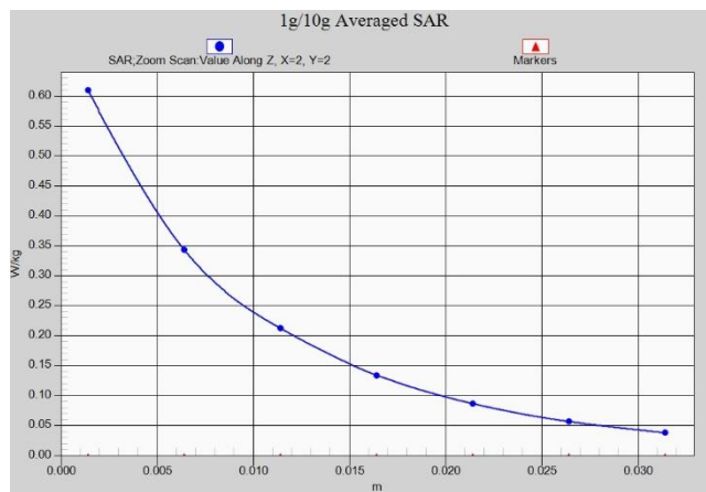
Fig. 1-17 Z-Scan at power reference point (LTE Band5)
