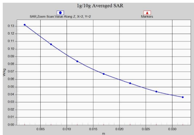
Fig. 1-23 Z-Scan at power reference point (LTE Band17)
