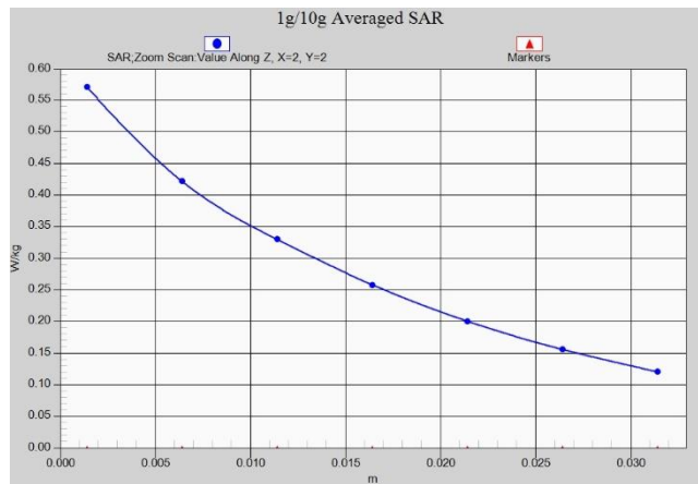
Fig. 1-12 Z-Scan at power reference point (WCDMA850)
