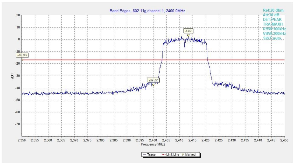
Fig.A.5.3 Band Edges (802.11g, Ch 1)
