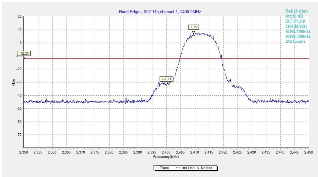
Fig.A.5.1 Band Edges (802.11b, Ch 1)
