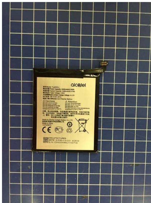
Pic A-7 Label of Battery AE2(CAC240006CJ)
