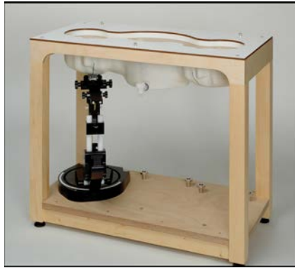
Picture C.10: SAM Twin Phantom
