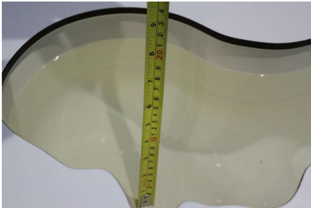
Picture 7-7: Liquid depth in the Head Phantom(5GHz)
