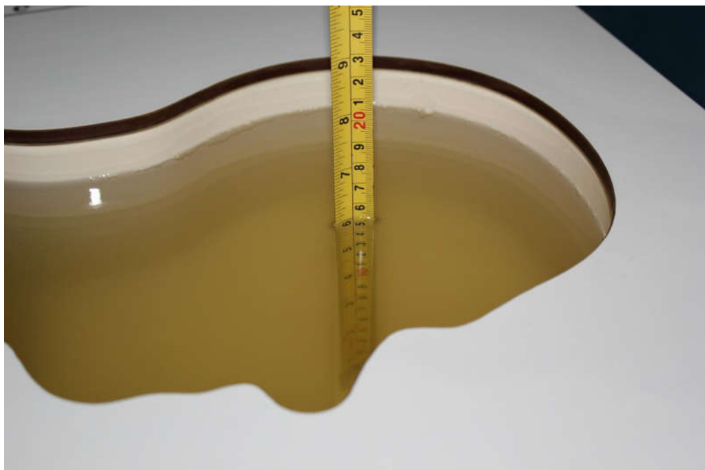
Picture 7-6: Liquid depth in the Head Phantom(2550MHz)
