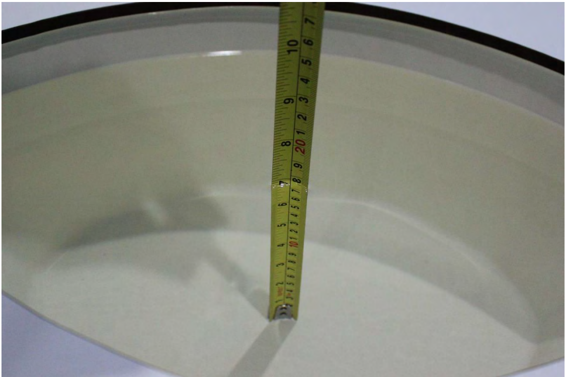
Picture 8-9 Liquid depth in the Head Phantom (5GHz)
