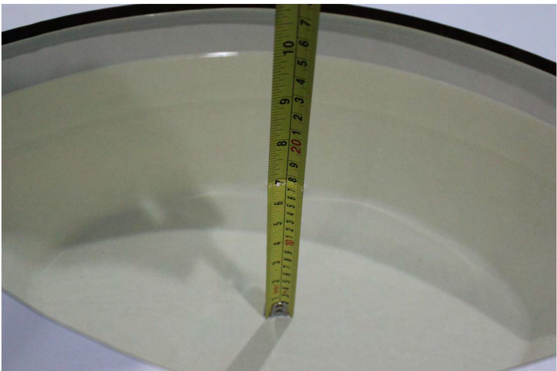
Picture 8-8 Liquid depth in the Head Phantom (3900 MHz)
