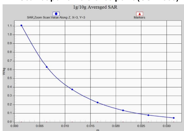
Z-Scan at power reference point (GSM1900)
